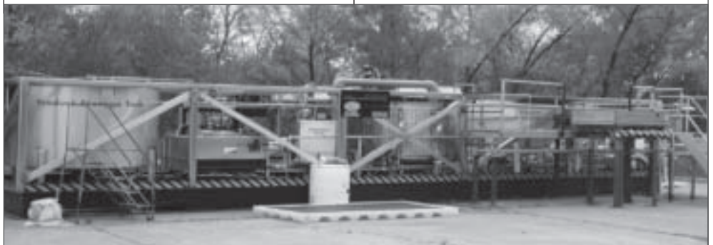
Transportable Propellant Conversion Unit (U.S. Army photo.)
