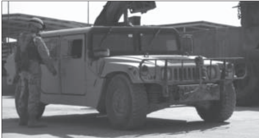
Although ASKs provide increased survivability to deployed Soldiers, the kits cause temperatures inside Humvees to rise to more than 100 degrees fahrenheit. TARDEC is developing a cooling system to solve this problem. (U.S. Army photo by SPC James Smith.)
