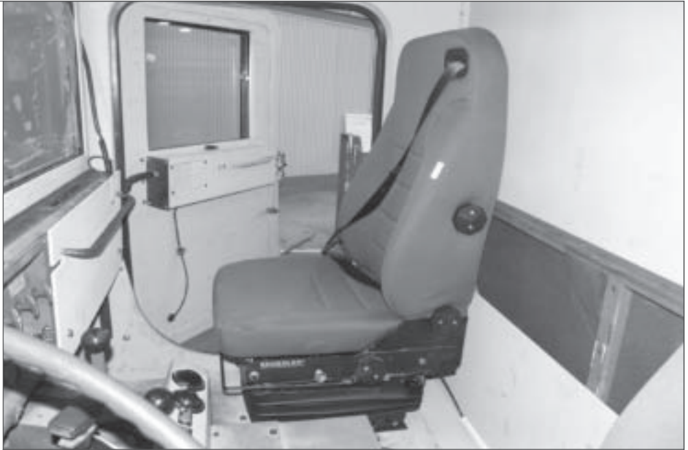
Bench seats were removed and new air ride bucket seats were installed to accommodate the gunner platform and A/C unit. In addition, power actuators were installed to assist in moving the heavy doors along with a powered assembly that moves the side transparencies up and down. (U.S. Army TARDEC photo.)
