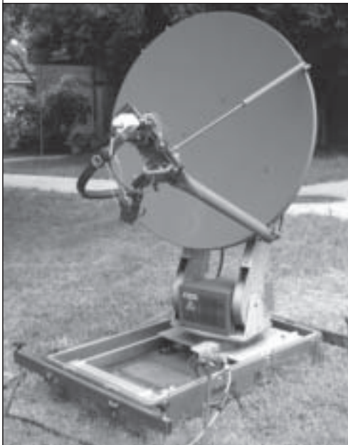
Shown here is the new model of the CSS VSAT satellite communications system, featuring a slightly larger antenna dish — a 2-piece dish with interlocking connections that is 1.2 meters in diameter, compared to .96 meters for the prototype. That small increase allows for greater beam coverage and means less rain-fade degradation, which translates into better performance.
