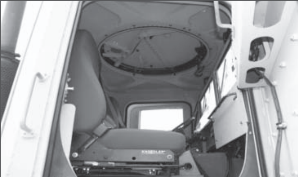
TARDEC engineers fitted the M939 up-armored cab with a Humvee lightweight gun ring. (U.S. Army TARDEC photo.)
