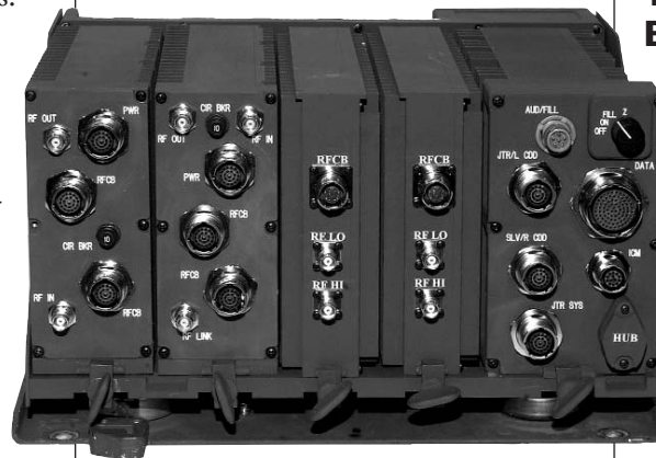
The JTRS Cluster 1 participated in the PSV automated pilot program. The JTRS Cluster 1 provides the warfighter with a software-reprogrammable, multiband/multimode capable, networkable system that provides simultaneous voice, data and video communications.
