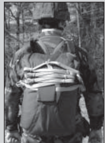
The MC6 system rigged on the jumper ready for use. The MC6 system consists of the ATPS harness and pack tray, ATPS reserve personnel parachute and SF-10A main canopy. The outside appearance of the SOFTAPS and ATPS is the same with the exception of the blue nylon webbing used for the confluence wrap on the risers, which allows for easy recognition of systems at the time of issue from the parachute storage/issue facility. The ATPS will replace the MIRPS.
