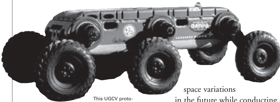
This UGV prototype is designed for endurance, obstacle negotiation and transportability. These prototypes may include unique mobility configurations (traditional wheeled/tracked to organic-mimicking, i.e., walking/crawling), exceptional drive trains, advanced structures and composites, terrain and soil analysis, sensory exploitation and interaction with robotic control architectures.
