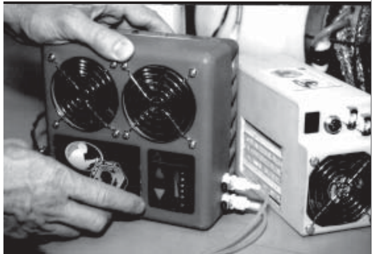
Two working personal cooler prototypes weighing less than 5 pounds have been developed in the latest step to downsizing the system.
