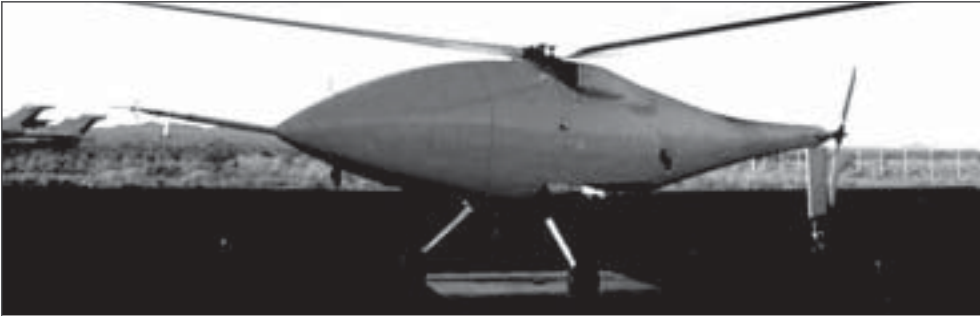
The A160 Hummingbird is a UAV with VTOL ability. The A160 concept is being evaluated for surveillance and targeting, communications and data relay, lethal and non-lethal weapons delivery, assured crew recovery, resupply of forces in the field and special operations missions in support of Army, Navy, Marine Corps and other DOD needs. It is being developed as a DARPA/Army FCS Program component.
