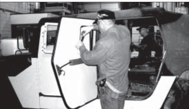
TARDEC engineers install an ASK on a HMMWV at APG prior to field testing.
