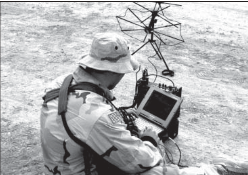
SPC Philip Amiot, 82nd Airborne Division's Long Range Surveillance Detachment, uses an AN/PSC-5 Spitfire UHF Manpack Terminal and a laptop computer to send still images to satellites. Amiot is taking part in a live-fire exercise at a range outside of Bagram Airfield, Afghanistan. U.S. Army photo by SPC Jeremy Colvin, 55th Signal Co.
