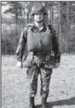
The MC6 system rigged on the jumper ready for use. The MC6 system consists of the ATPS harness and pack tray, ATPS reserve personnel parachute and SF-10A main canopy. The outside appearance of the SOFTAPS and ATPS is the same with the exception of the blue nylon webbing used for the confluence wrap on the risers, which allows for easy recognition of systems at the time of issue from the parachute storage/issue facility. The ATPS will replace the MIRPS.
