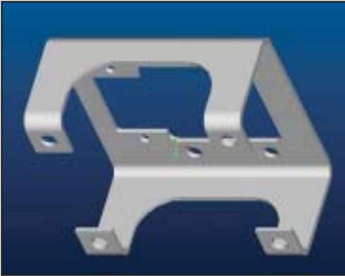
Figure 2. A sample 2-D CAD drawing of a relay-circuit breaker box bracket from the M113 FOV that was converted to a parametric 3-D model.
