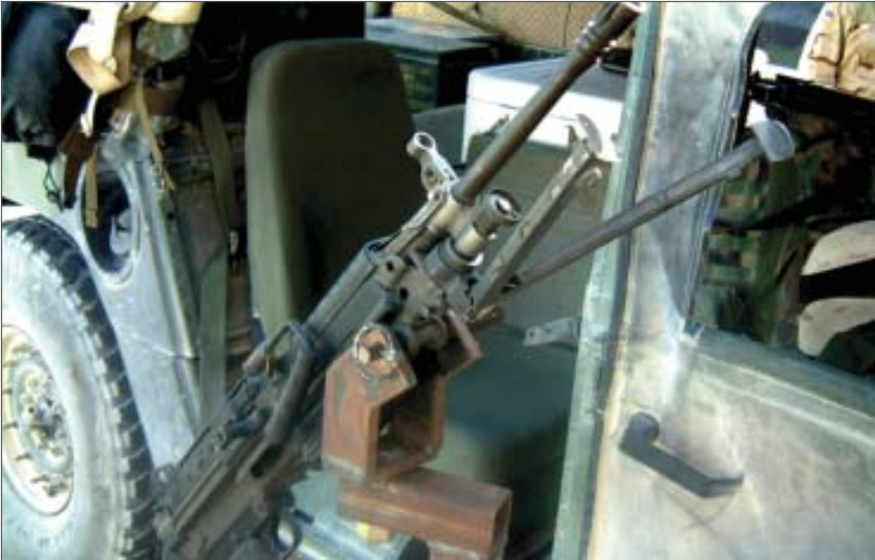
The MPH RMS team manufactures pintle assemblies and attaching locking pins for 5.56mm SAW gun mounts on HMMWVs. These gun mounts allow a 180-degree turning radius.
