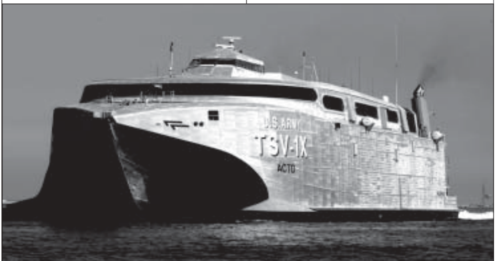
The TSV-1X, shown above, is one of two high-speed catamarans being tested as a logistics support platform as part of the Army's transformation plan.
