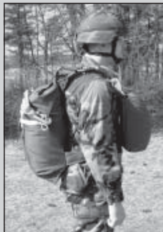
The MC6 system rigged on the jumper ready for use. The MC6 system consists of the ATPS harness and pack tray, ATPS reserve personnel parachute and SF-10A main canopy. The outside appearance of the SOFTAPS and ATPS is the same with the exception of the blue nylon webbing used for the confluence wrap on the risers, which allows for easy recognition of systems at the time of issue from the parachute storage/issue facility. The ATPS will replace the MIRPS.
