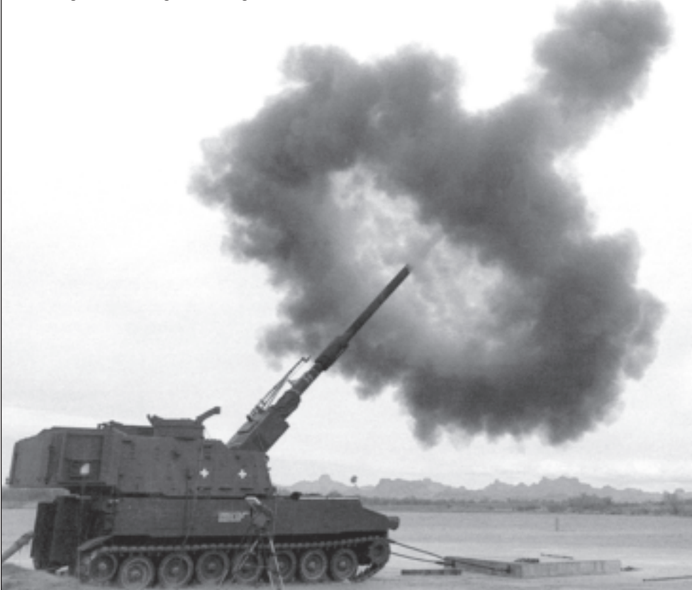
An Excalibur test projectile is being fired from a Paladin gun tube during field testing.
