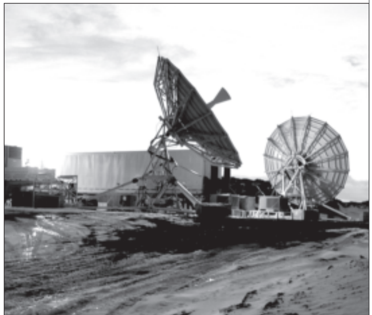
When the MDA accelerated its testing schedule and required a long-haul connection by April 1, 2004, PM DSCS-T provided, as an alternative, a new "D" version of an AN/TSC-86 terminal — with dual 20-foot diameter AS-3199 antennas to transmit and receive two satellite areas simultaneously.
