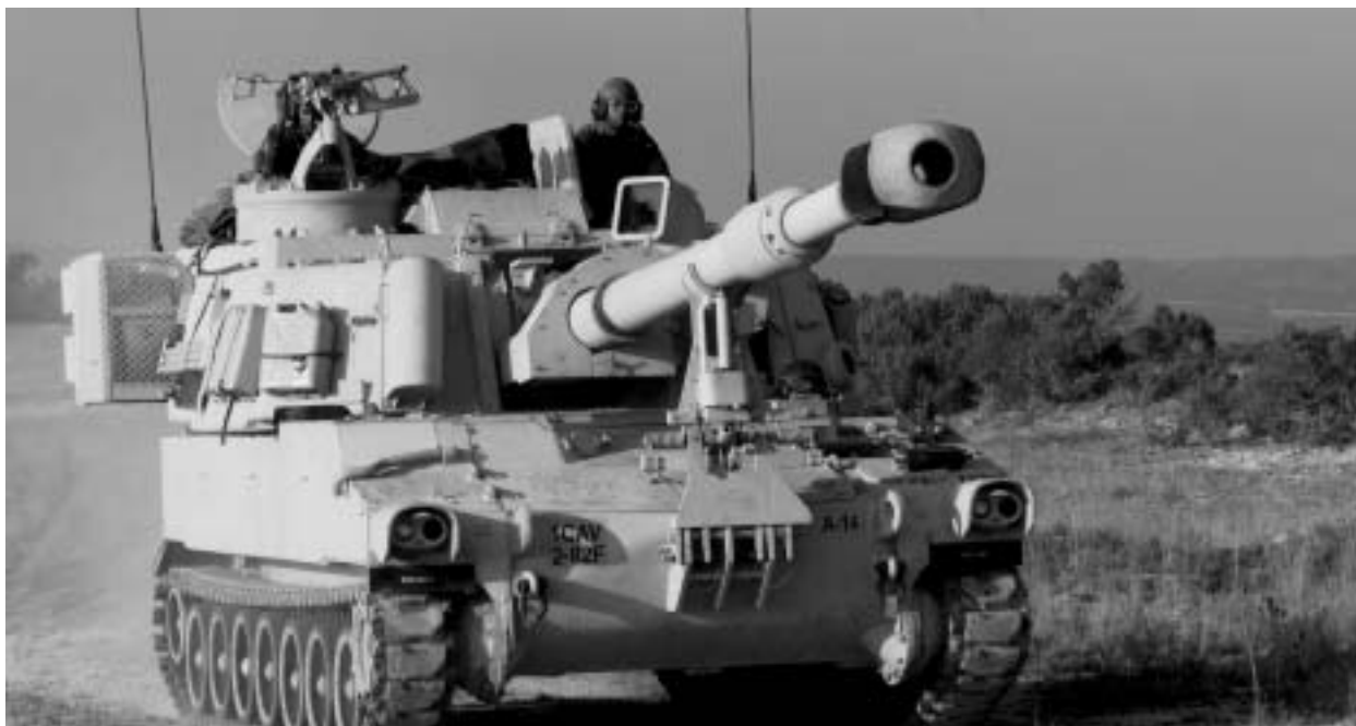
The Paladin uses an onboard computer system to receive fire missions, compare firing data, select and take up firing positions, automatically unlock and point its cannon, and then fire.
