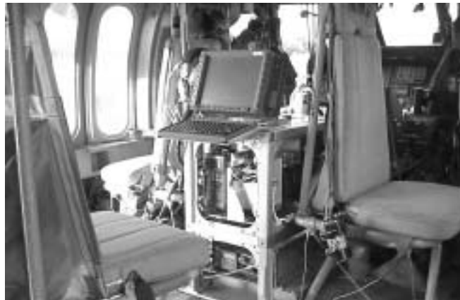
Photo depicts a Blue Force Tracking Aviation System installed in UH-60L Black Hawk helicopter.
