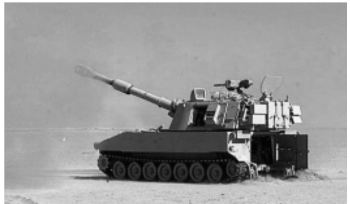
The M109A6 Paladin is a 155mm self-propelled howitzer, equipped with automated fire control, communications, and navigation systems.
