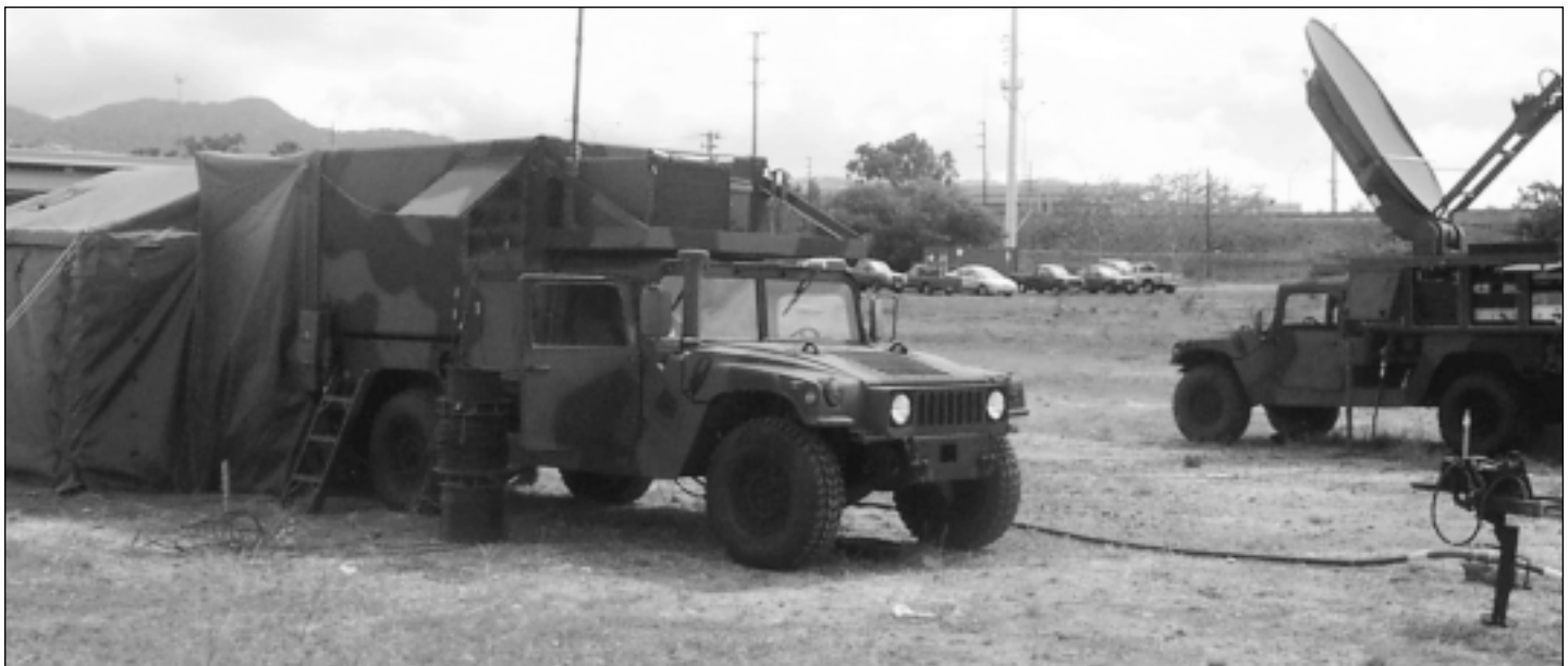
The deployable C4I Package includes the BBN (left vehicle) supported by a Tri-band Tactical Satellite Terminal (right vehicle).
