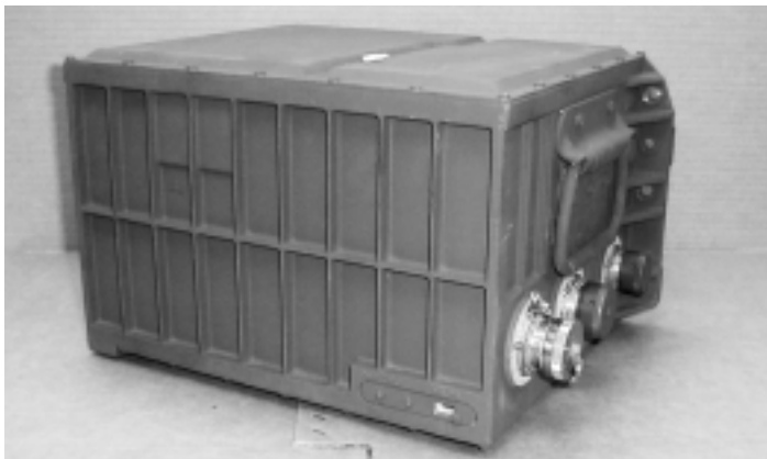
The DRU-H provides continuous position and pointing data to the M109A6 fire control computer.
