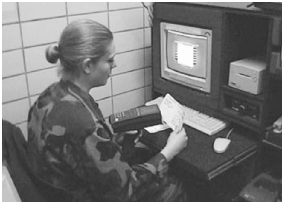
A soldier works with the Automated Manifest System, which takes source data from a Standard Army Management Information System and writes to AIT media (2-D bar code, optical memory card, and RF tag).
