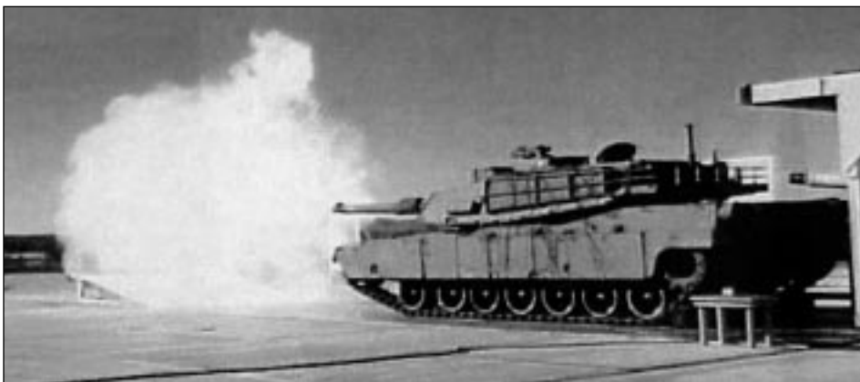
An M1A2 Abrams fires a 120mm projectile during an ammunition production acceptance test at the Red Bluff Firing Range at YPG.
