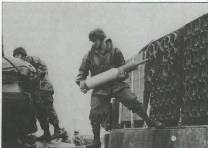
Soldiers load 120mm ammunition directly from improved containers on a HEMTT onto an M1A1 tank without breaking pallet banding.
