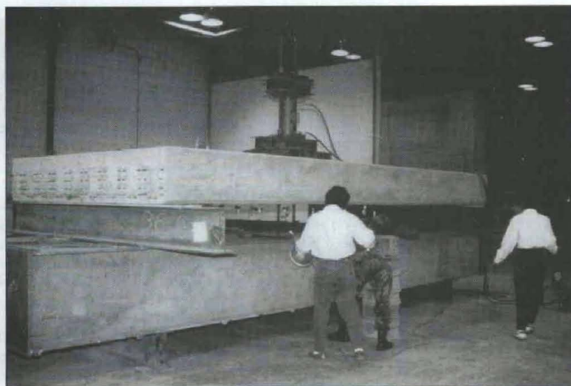
Laboratory test loading of the deck section made using carbon fiber reinforced composite cables.
