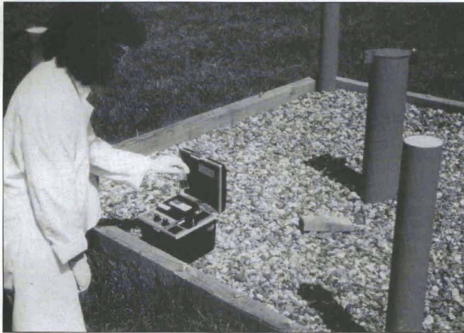
CRREL developed methods for near real-time determination of TNT contamination in soils have been commercialized by EnSys Inc. as a field test kit.
