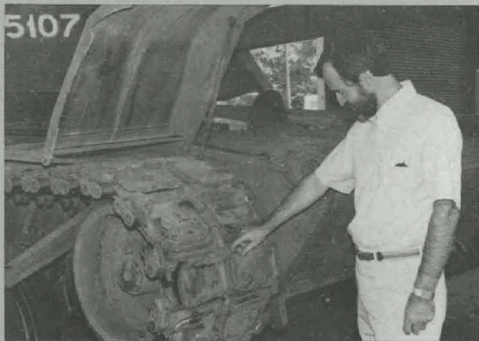
Ted Wheeler, M1 tank team leader, inspects the rubber pads on an M1 Abrams tank.
