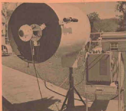
CASSEGRAIN SYSTEM with 20-inch diameter receiver picks up signals from distance of 400 feet in daylight.
