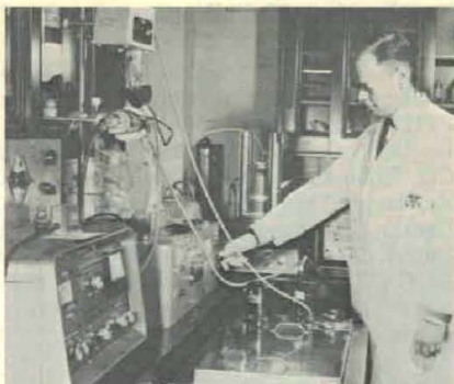
EQUIPMENT for measuring radioactivity from chromatographic column is used in physiologic experiments.
