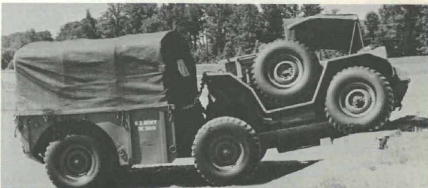
"GAMA GOAT" climbs up and over walls and obstructions as high as 18 inches and has a flexibility of 18 special uses. The vehicle can carry a crew of 10.
