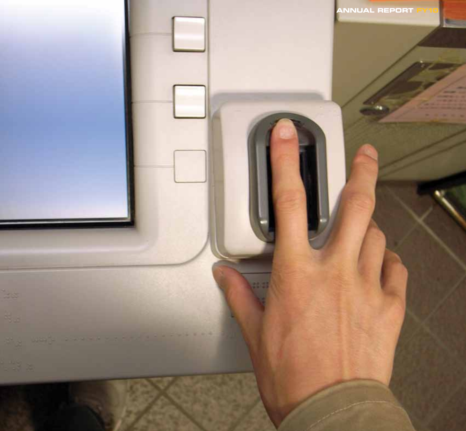
Finger vein technology as used for secure access to an ATM. (Source: flickr/Matsuyuki)
