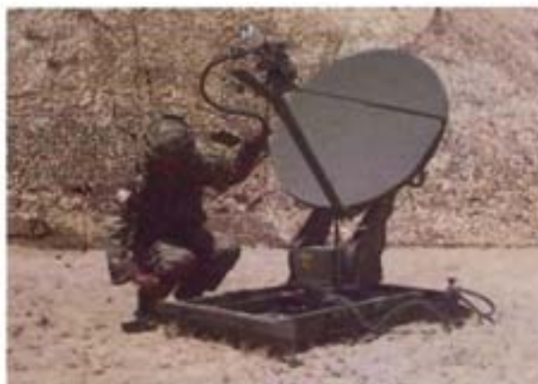
Image 01. A soldier adjusts outriggers on a Very Small Aperture Terminal (VSAT) satellite system. (Photo Courtesy of U.S. Army/Mike Kane.)
