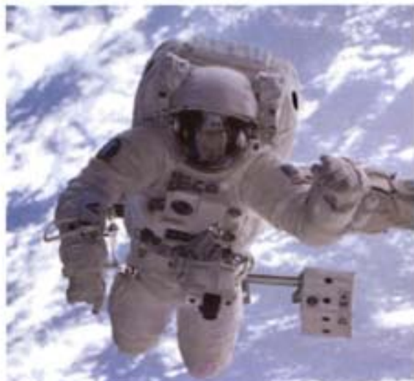
Image 14. A NASA spacesuit consists of 14 layers of nylon tricot, spandex, urethane-coated nylon, dacron, neoprene, aluminized mylar, gortex, kevlar, and nomex. (Photo Courtesy of NASA / 1995.)
