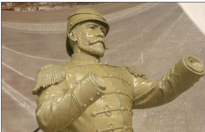
The John Philip Sousa statue undergoes a process of layering liquid rubber over a clay base on Aug. 18, 2005 at Laran Bronze Foundry in Chester, Pa.
