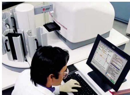
A technician reads results from the automated, scalable SNPstream genotyping system, which includes a robotic analysis instrument and computer readout.
