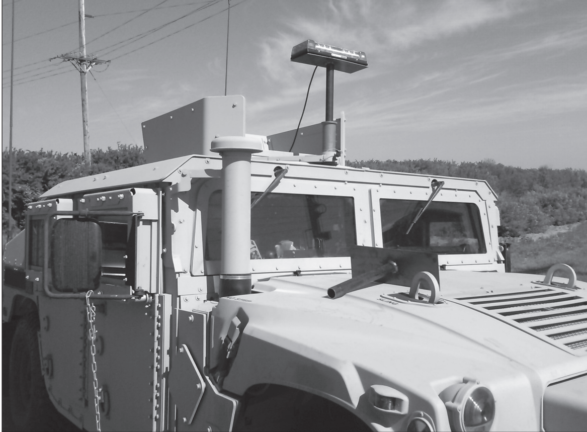
Modified mounting bracket and detachable light bar on a Humvee
