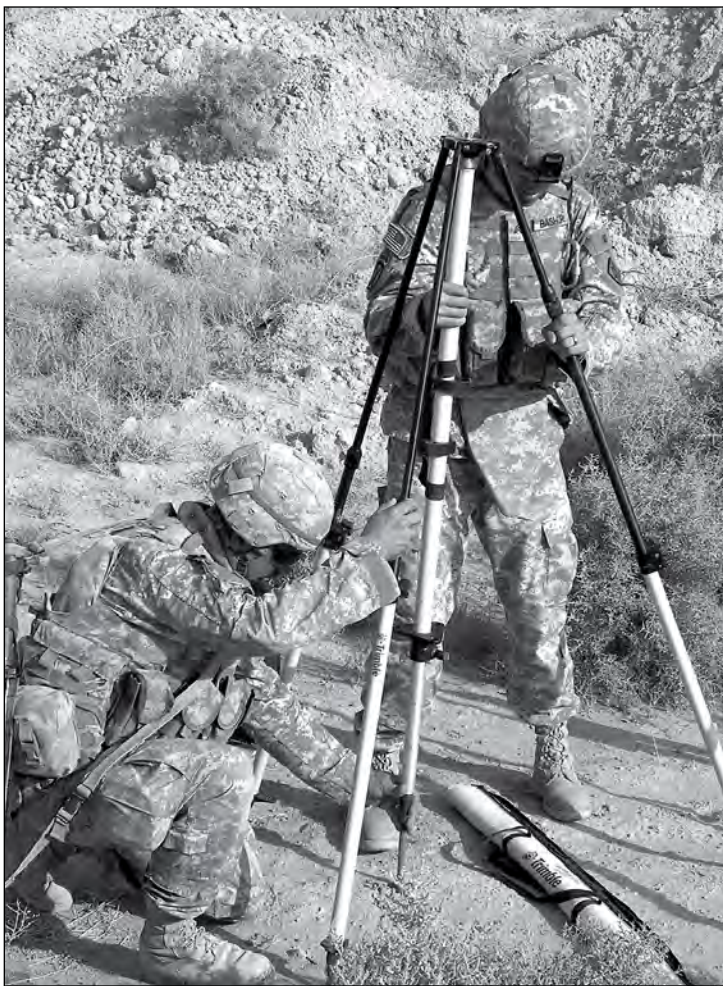
Personnel from the 243d Construction Management Team set up a surveying beacon near Patrol Base Dragon in Iraq.
