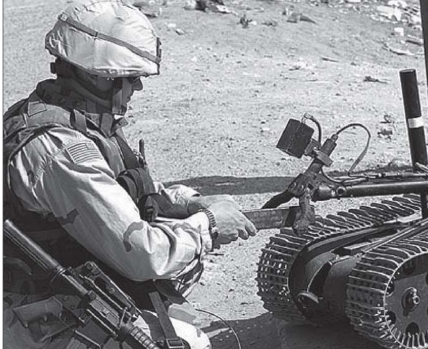
A Soldier prepares a TALON robot for use during a route clearance patrol.
