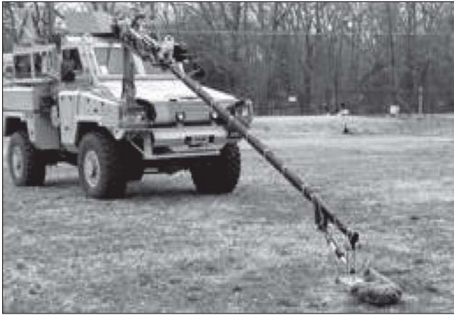
A prototype of an RG-31 with an arm investigates a suspicious object during testing.
