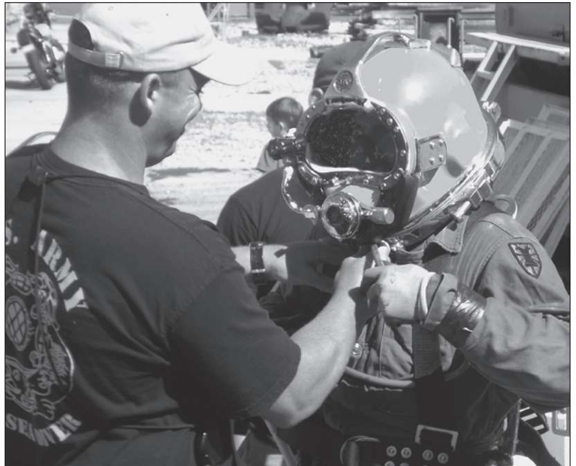
A dive supervisor inspects a surface-supplied diving helmet before deploying a diver into the water to remove debris from under a boat lift.
