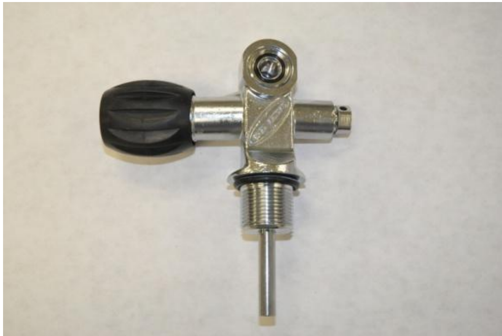
Figure 8. Front view of the exemplar cylinder valve. The valve stem assembly and housing is concealed by the black valve handle.
