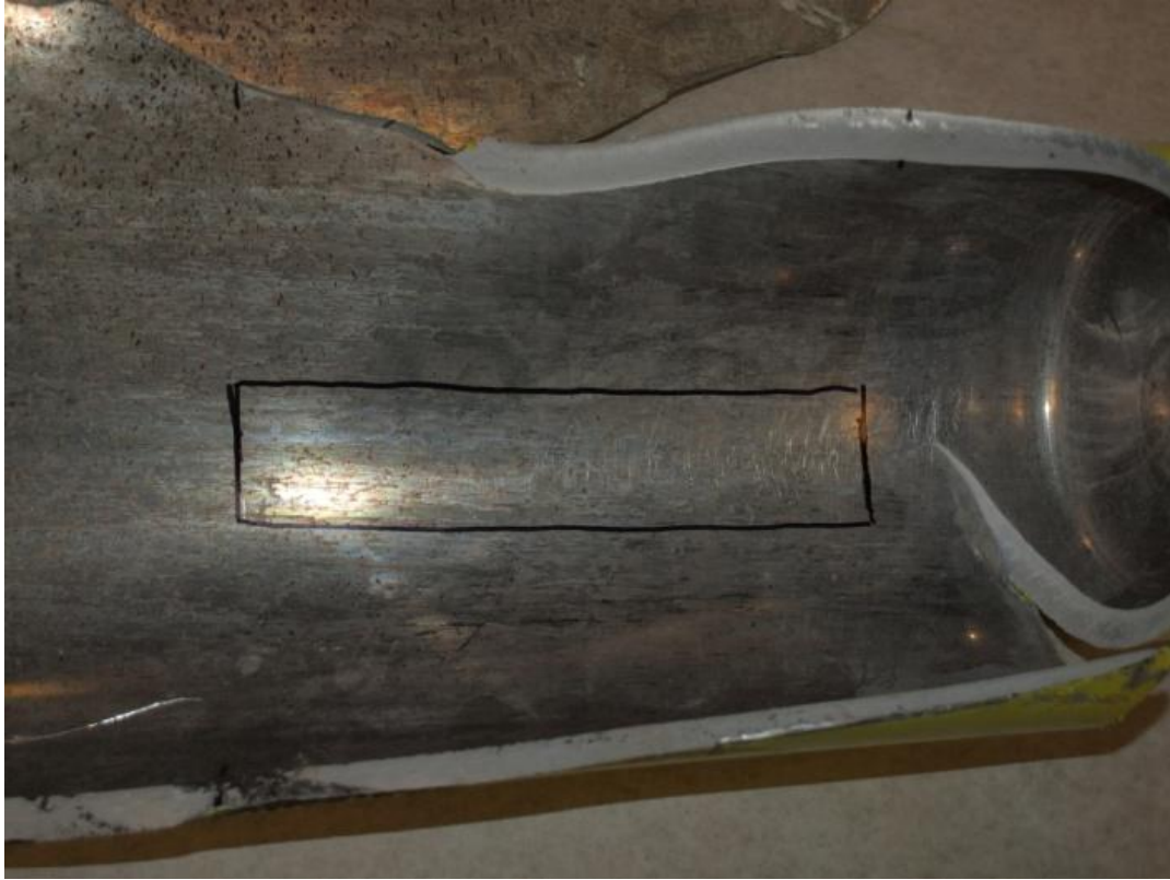
Figure 28. View of the incident cylinder showing the location of the billet removed for machining into tensile and compressive test specimens.
