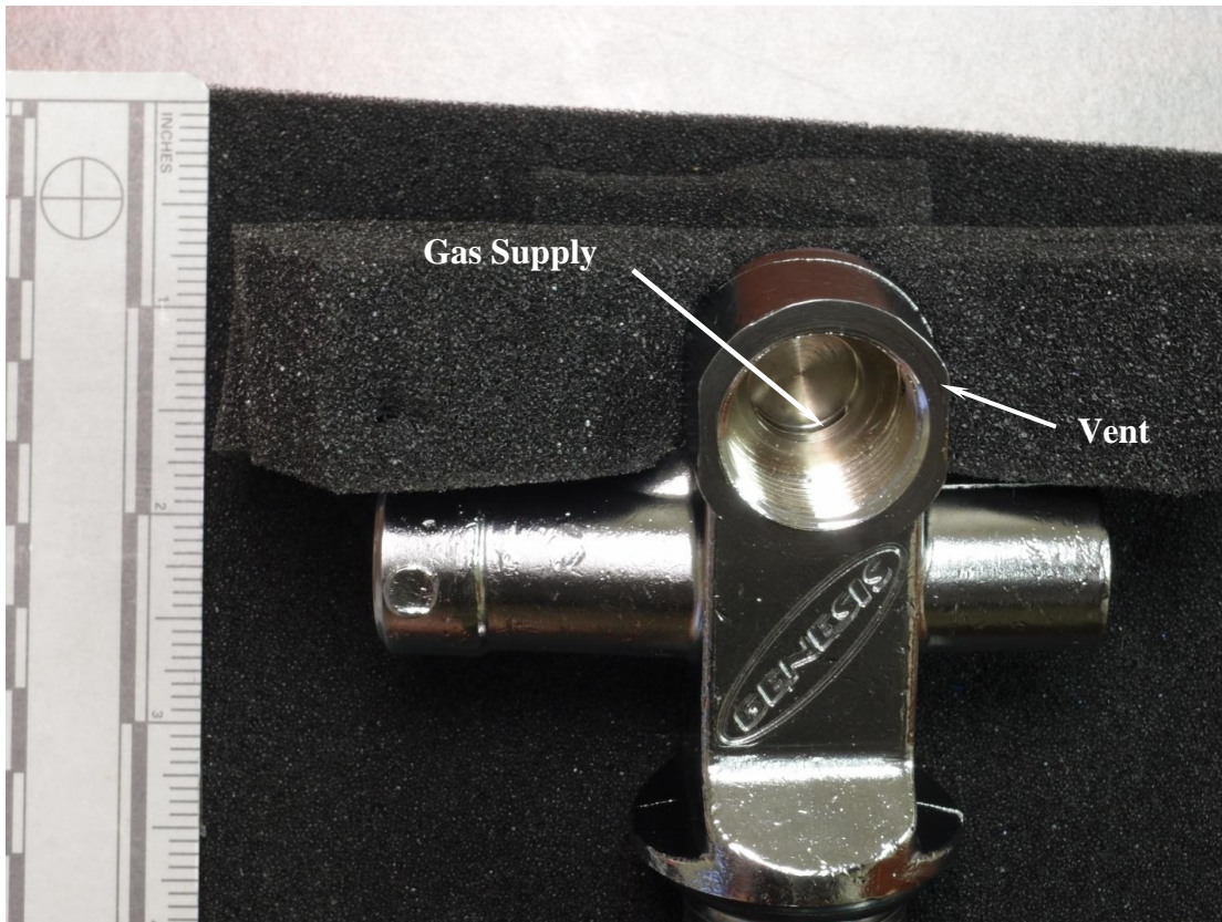
Figure 13. Front view of the exemplar cylinder valve showing the high pressure regulator port.
