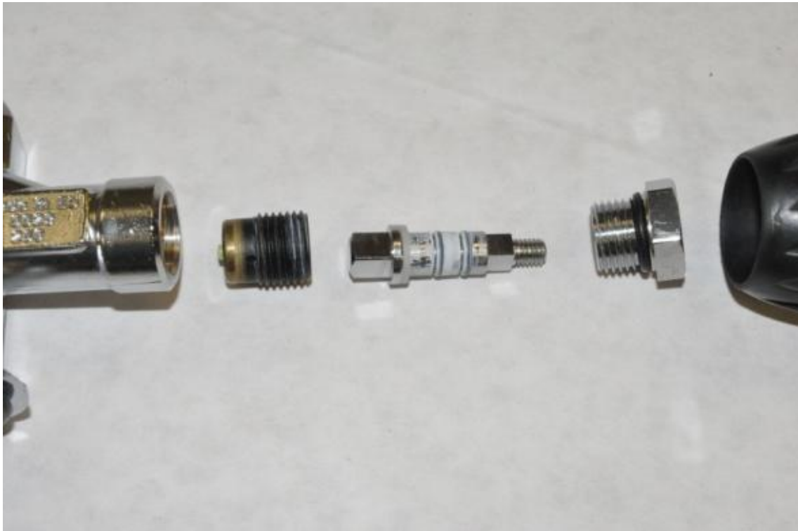
Figure 10. Rear view of the fully disassembled exemplar valve stem assembly showing the valve seat body and its orientation in the assembly.
