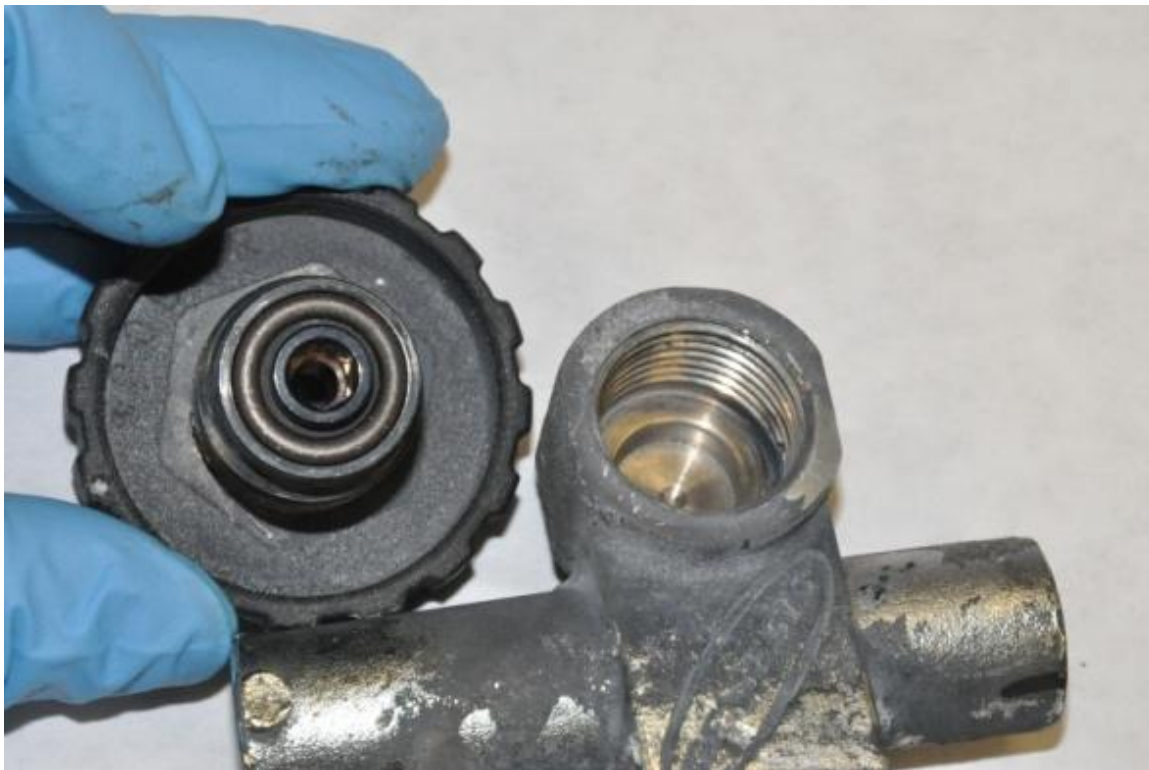
Figure 20. View of the incident valve and underside of the regulator adapter handle.
