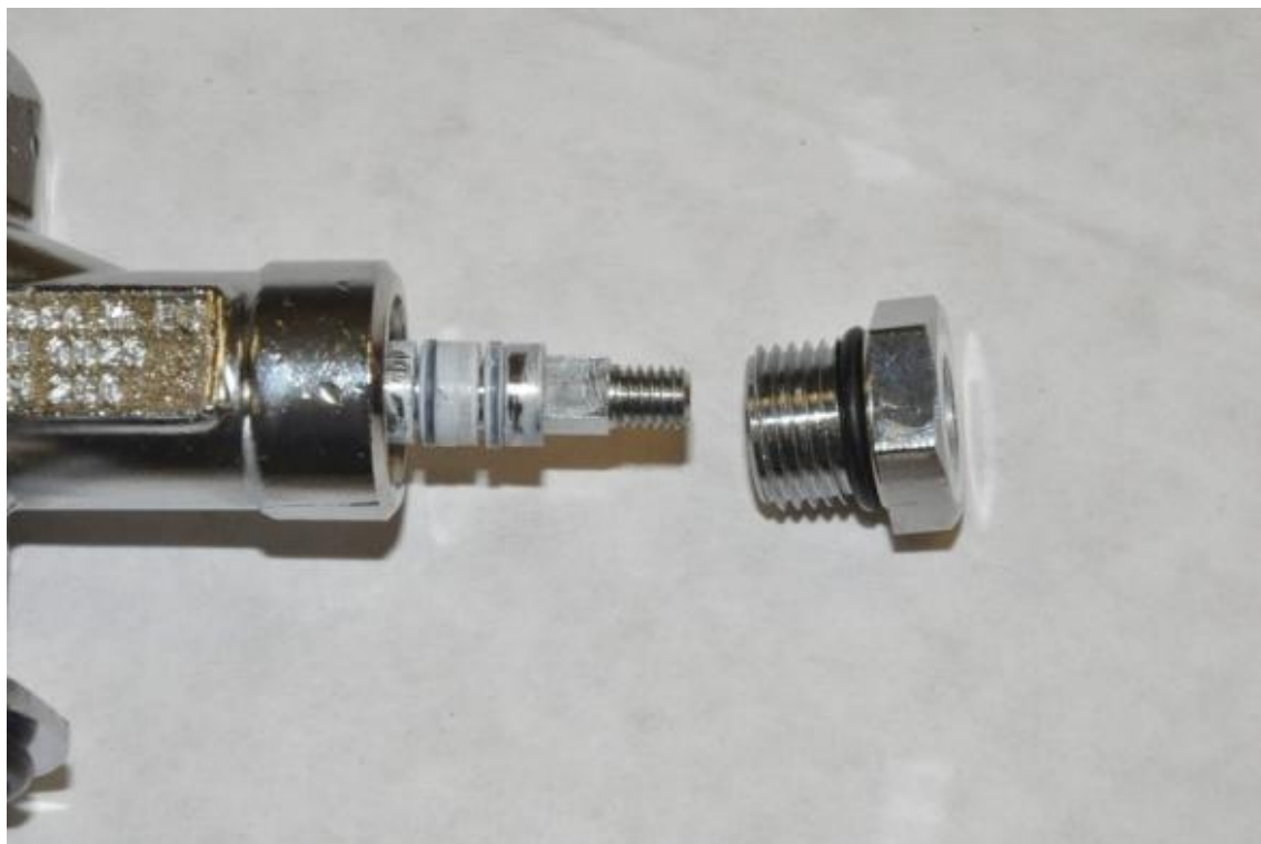
Figure 9. Rear view of the partial exemplar valve stem assembly showing the gland nut, O-ring, and valve stem.
