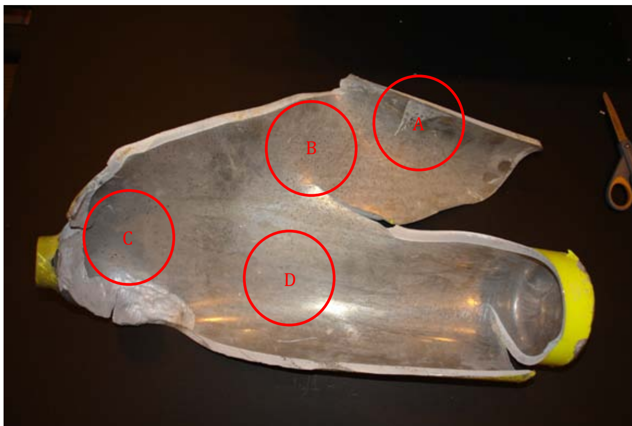
Figure 1. Solvent wash areas for FTIR sampling.
