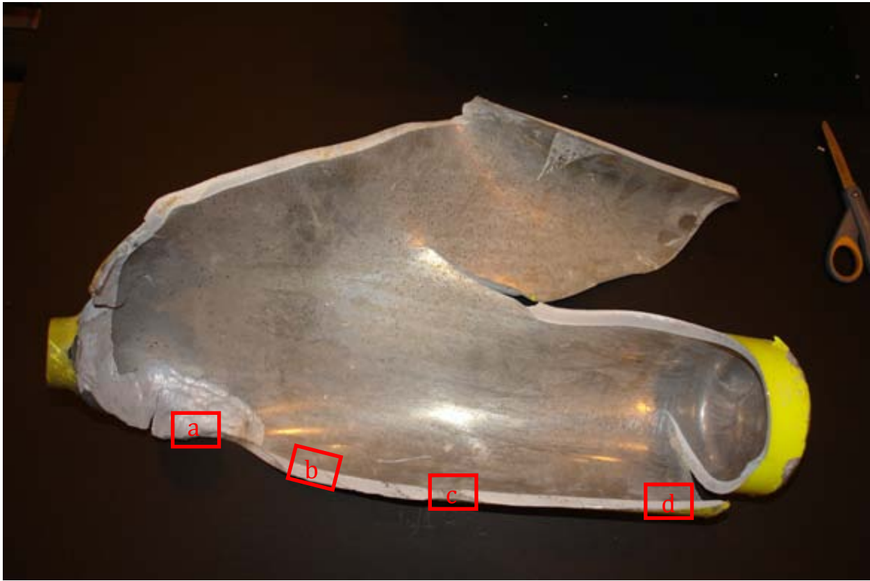
Figure 2. Approximate test sites for hardness testing and metallographic examination.
