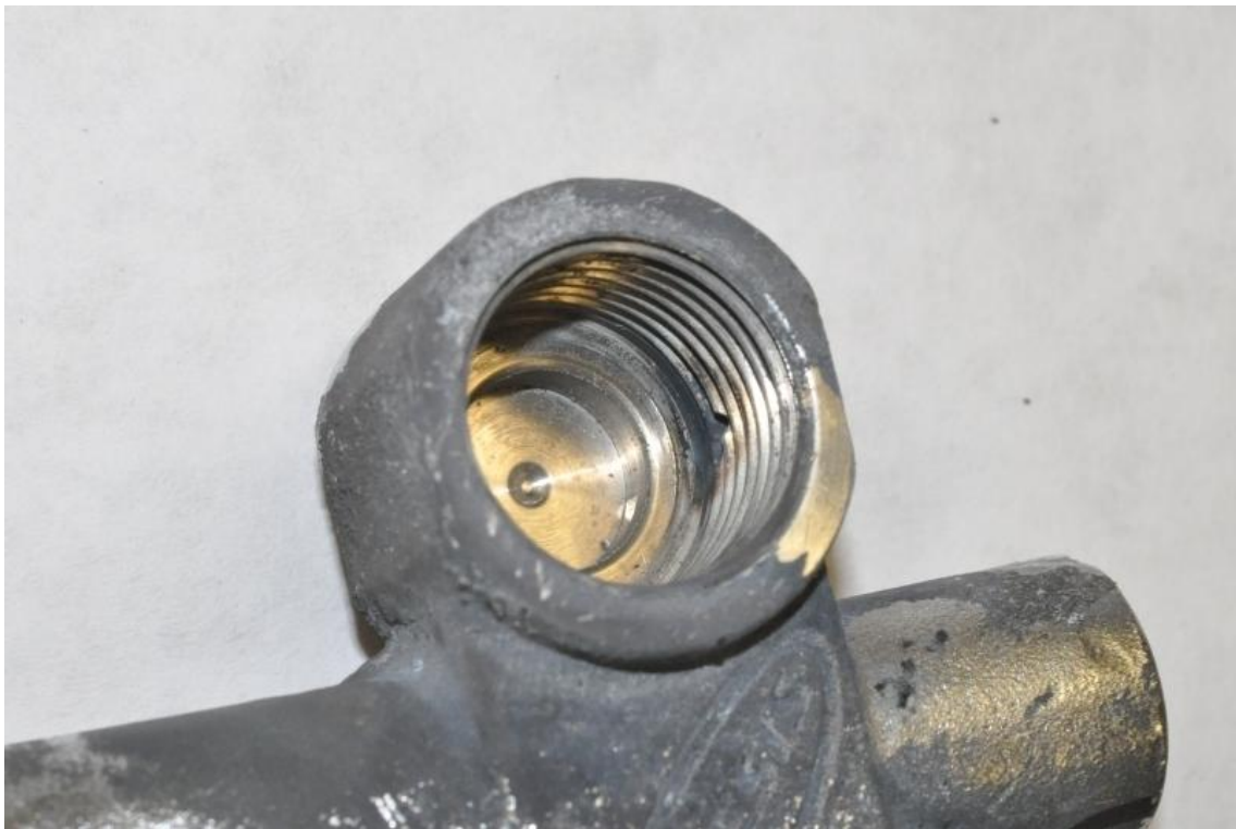
Figure 19. View of the incident valve high pressure regulator port showing discoloration sooting around the vent.
