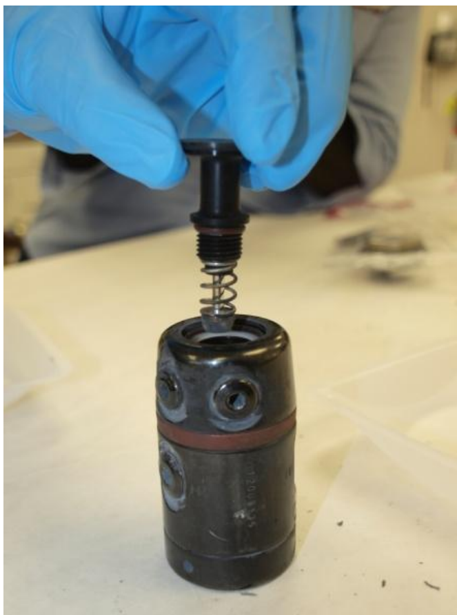
Figure 21. View of the incident regulator with the cap/spring/plunger assembly being removed.
