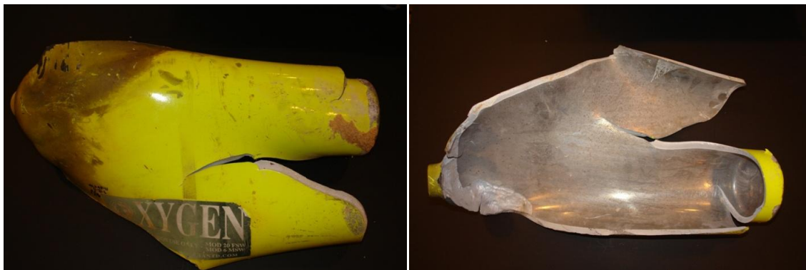
Figure 4. Larger portion of high pressure gas cylinder
