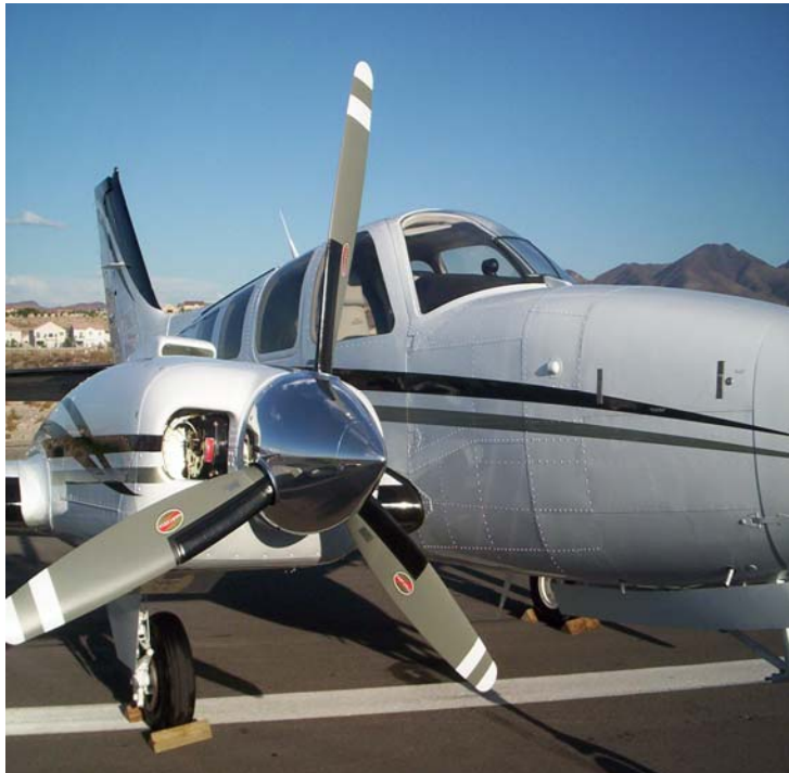
Aircraft certificated under Part 36 Subpart F "Propeller Driven Small Airplanes and Propeller-Driven, Commuter Category Airplanes" do not have a stage classification, and as such are referred to as nonstage. Most small general aviation aircraft and many commuter aircraft are nonstage aircraft. An example is the Beechcraft 58 Baron. (Photo: FAA)
