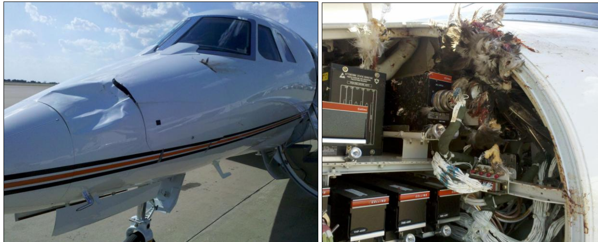
A Cessna 560 on final approach to an airport in Texas hit a large raptor at 2,400 feet on 27 July 2011, causing damage to nose and fuselage. Photo, M. Gardner.
