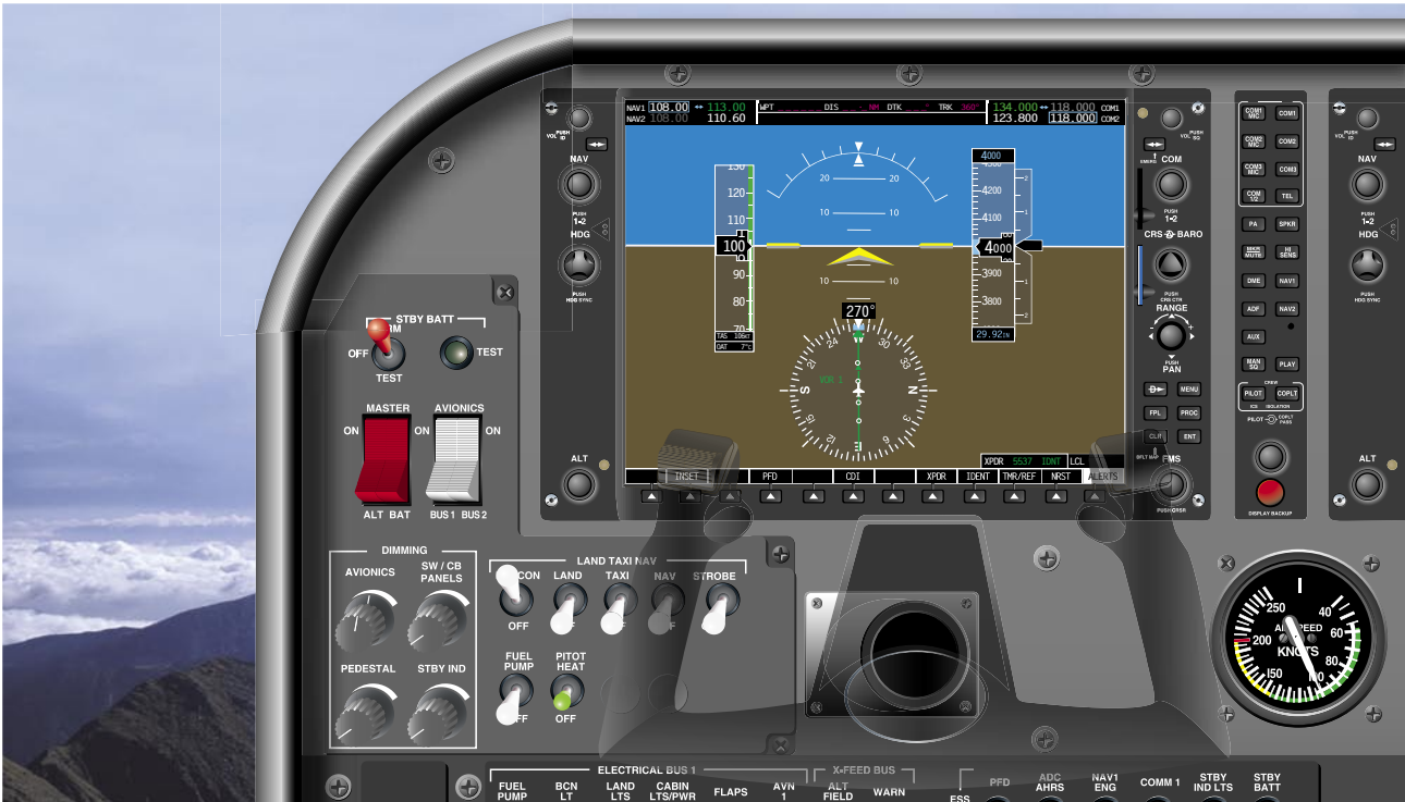
Figure 17-19. Two similar flight decks equipped with the same information two different ways, analog and digital. What are they indicating? Chances are that the analog pilot will review the top display before the bottom display. Conversely, the digitally trained pilot will review the instrument panel on the bottom first.
