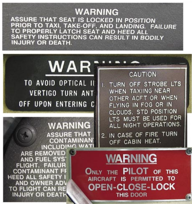
Figure 8-5. Placards are used to depict aircraft limitations.
