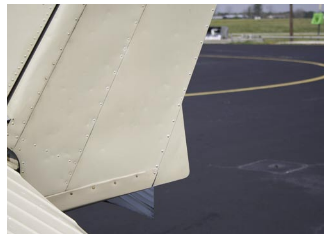
Figure 5-22. A ground adjustable tab is used on the rudder of many small airplanes to correct for a tendency to fly with the fuselage slightly misaligned with the relative wind.
