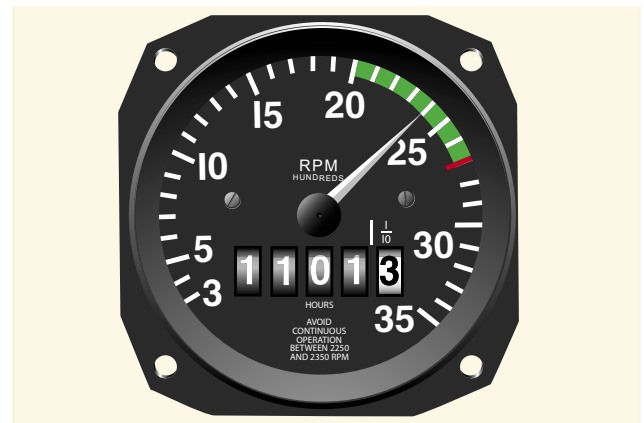
Figure 6-8. Engine rpm is indicated on the tachometer.
