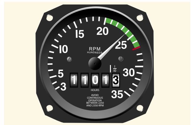
Figure 6-8. Engine rpm is indicated on the tachometer.
