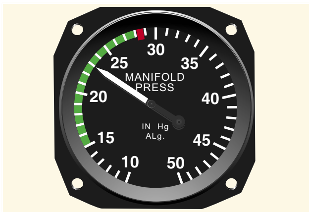
Figure 6-9. Engine power output is indicated on the manifold pressure gauge.
