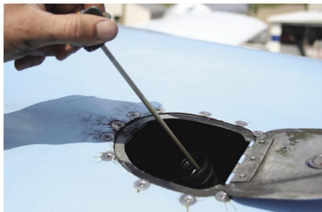
Figure 6-18. Always check the engine oil level during the preflight inspection.
