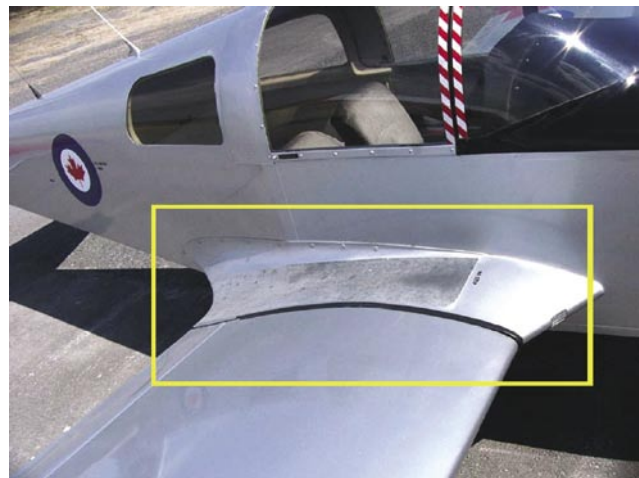
Figure 4-6. A wing root can cause interference drag.
