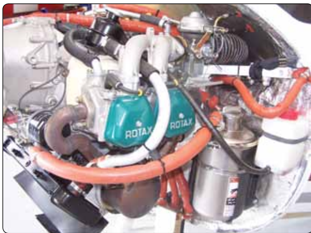
Figure 11-6. Typical four cylinder, four-stroke horizontally opposed engine.
