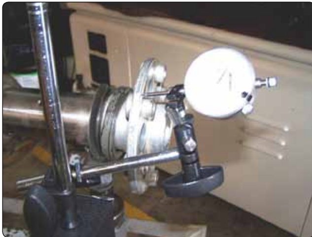
Figure 10-10. Checking crankshaft runout.
