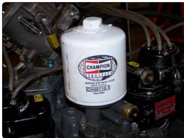
Figure 6-8. Full flow spin-on filter.
