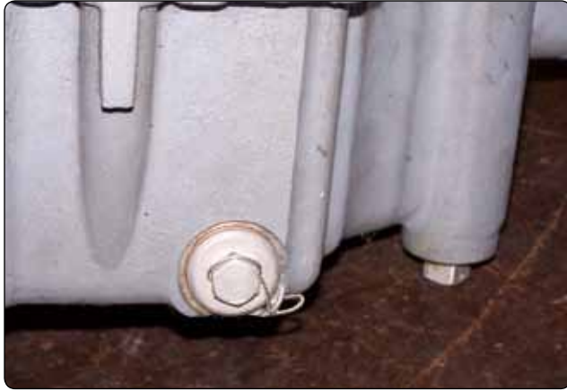
Figure 6-28. Oil sump screen.
