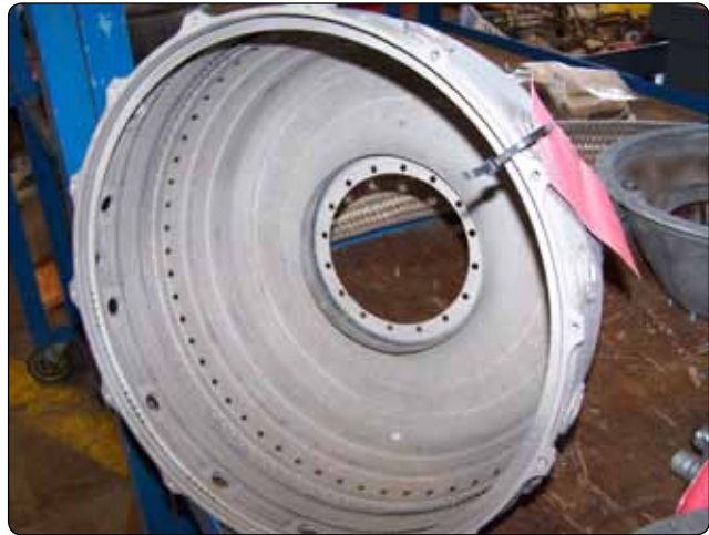
Figure 10-63. Combustion case inspection.
