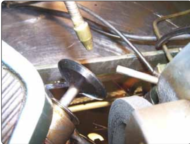
Figure 10-25. Valve in chuck ready to grind.
