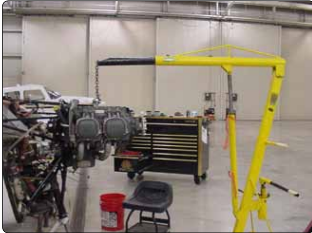
Figure 8-14. Relieve tension on engine mounts.
