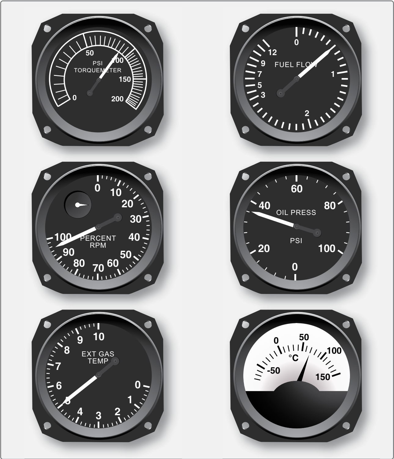
Figure 10-73. Typical turbine engine instruments.
