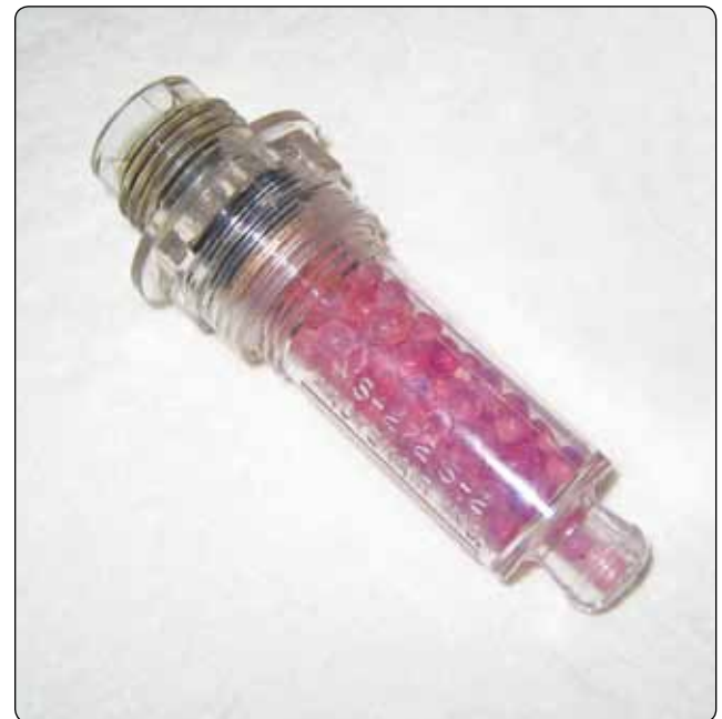
Figure 8-27. Dehydrator plug “pink” showing high humidity (Sacramento Sky Ranch).
