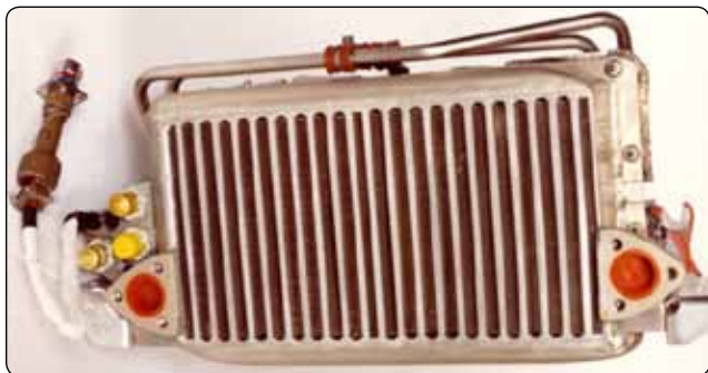
Figure 6-42. Air oil cooler.
