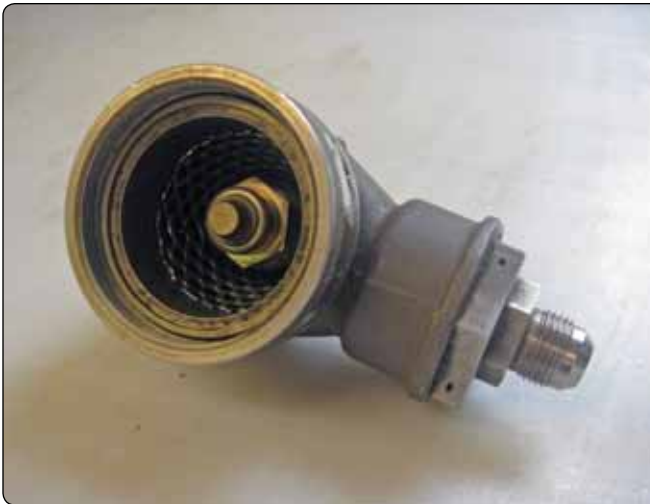
Figure 9-10. Discharge valve and cartridge (squib).
