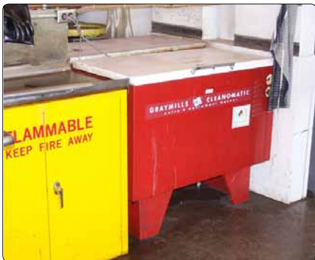
Figure 10-3. Typical solvent degreasing tank.
