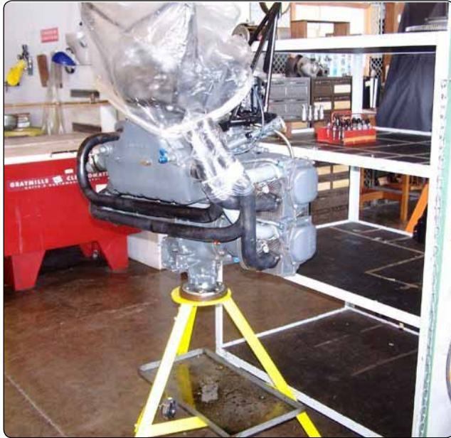
Figure 10-1. Engine mounted on an overhaul stand.
