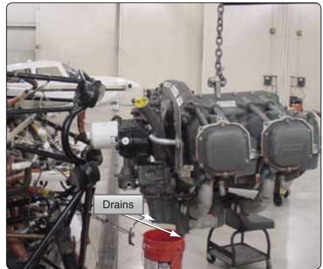
Figure 8-4. Oil system drain points.
