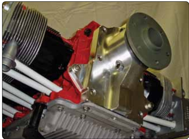
Figure 11-19. Front-end bearing on the 1000 IFB engine.
