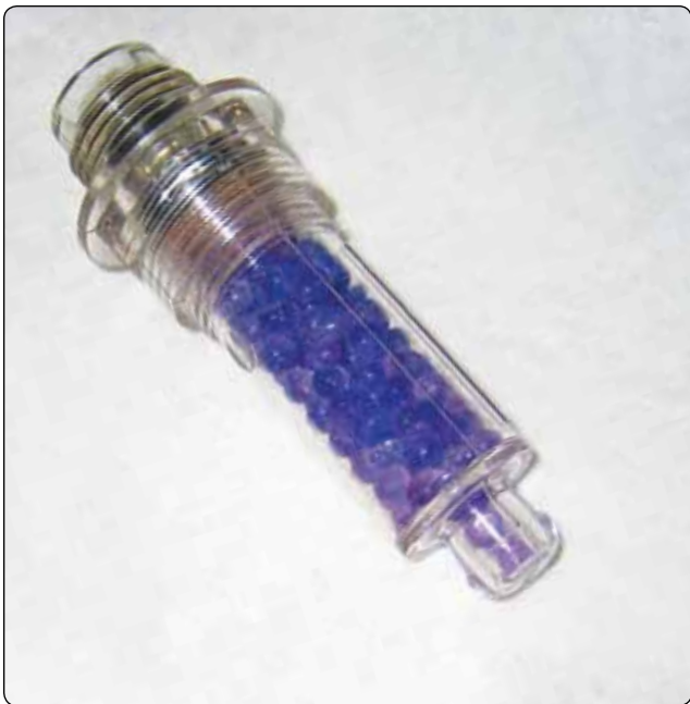
Figure 8-28. Dehydrator plug “blue” showing low humidity (Sacramento Sky Ranch).
