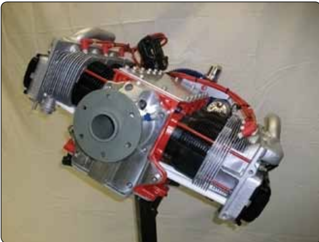
Figure 11-18. Aeromax direct drive, air-cooled, six-cylinder engine.
