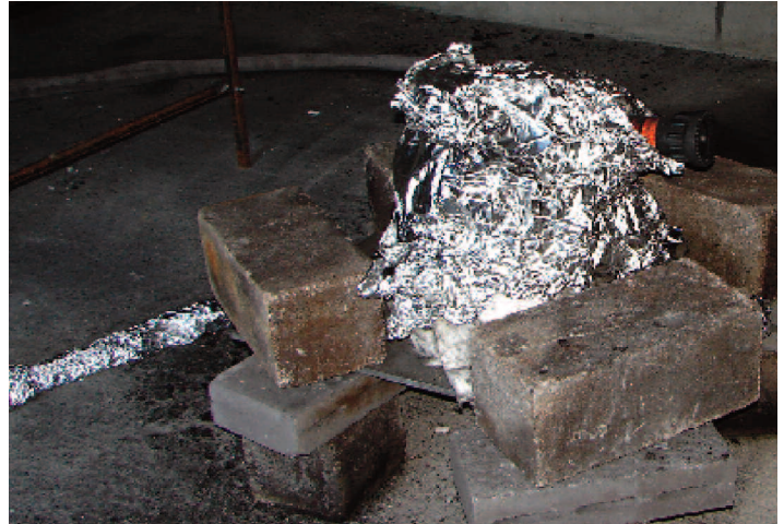
Figure 22: Remotely Controlled Fire Suppression Nozzle for Room and Contents Fires
