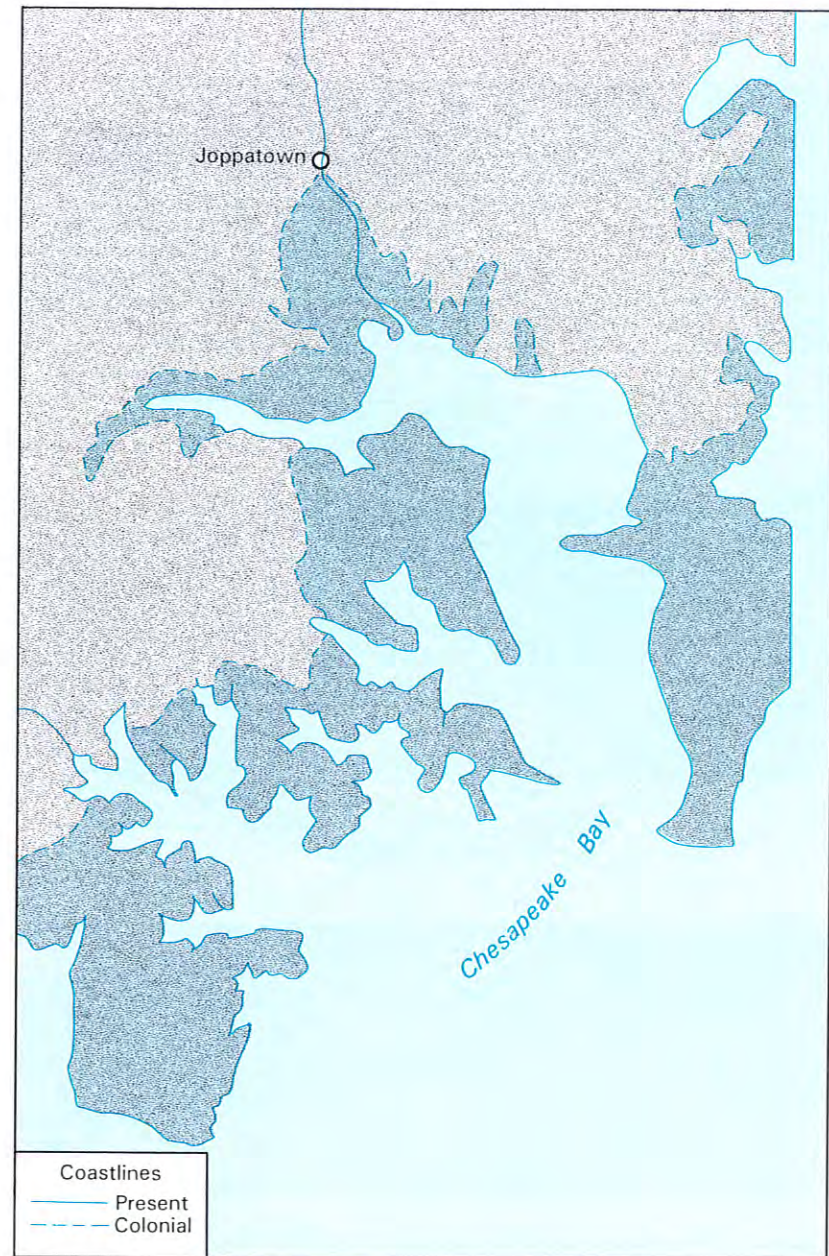
Figure 20. Poor land practices during Colonial times resulted in massive quantities of soil washing into nearby waterways, causing excessive sedimentation and fouling of navigable waters such as Joppatown harbor (EPA, 1989).
