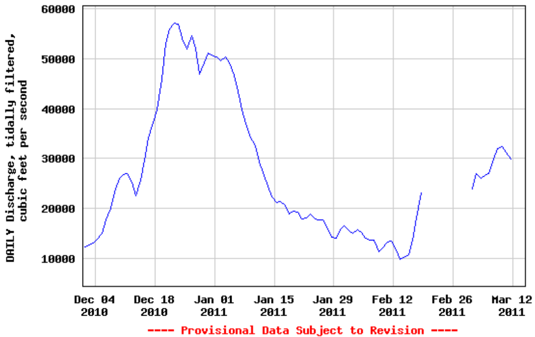
Figure 2. Tidally averaged Sacramento River flows measured at Rio Vista, December 1, 2010 through March 12, 2011.
