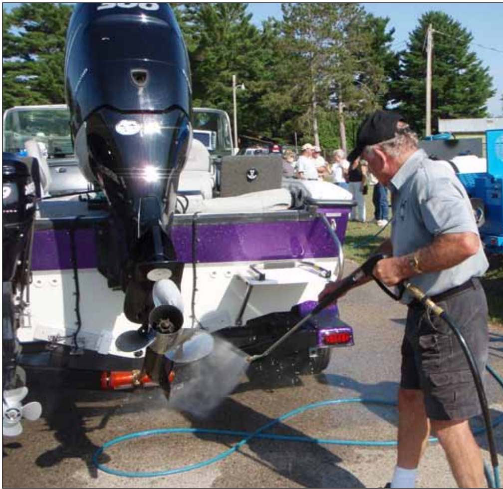
Wisconsin Deputy Conservation Warden Greg Stacey uses the power nozzle tool to decontaminate the transom. Note the blue mobile decontamination unit in the background. Photo courtesy of the Wisconsin DNR.
