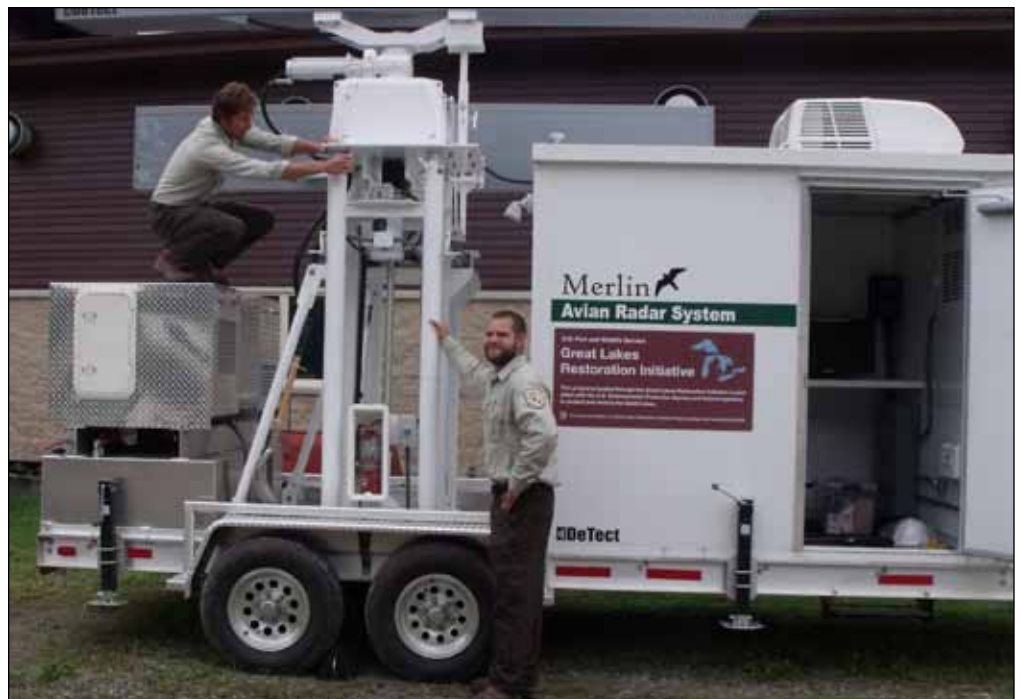
Avian Radar System (ARS) with Horizontal Scanning Radar antenna (top) deployed, Vertical Scanning Radar antenna (background) and GLRI logo.
