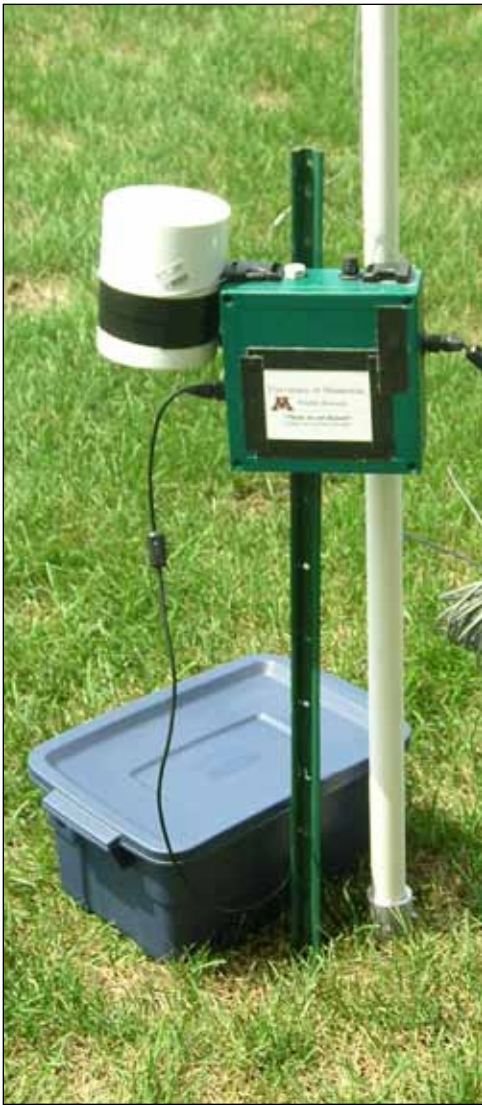
Close-up of the monitor (green box), battery (blue box), and ultrasonic microphone housing (white cylinder).
