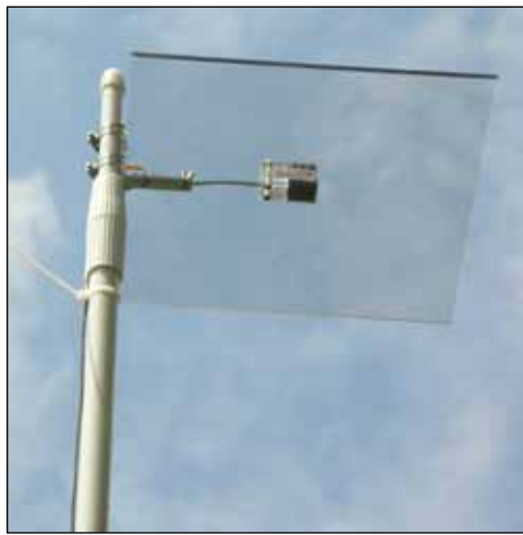
Acoustic microphone raised above ground to reduce ambient noise.
