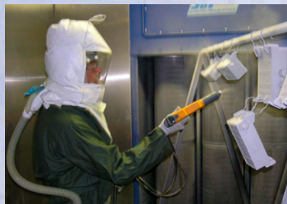
POWDER COATING IS AN EFFECTIVE, ENVIRONMENTALLY FRIENDLY PROCESS AT TAFB THAT DRASTICALLY REDUCES HAZARDOUS COMPOUNDS.
