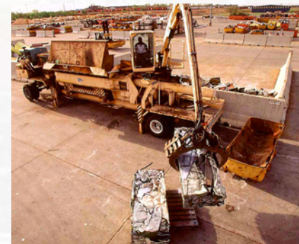
TAFB IS RECOGNIZED AS A PRIME ADVOCATE FOR RECYCLING MATERIALS. FINISHED BALES PRODUCE ONE-TENTH THE SCRAP METAL VOLUME COMPARED TO LOOSE SCRAP.
