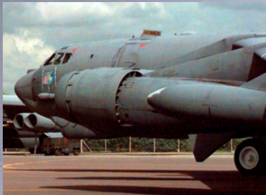
A SUCCESSFUL TF-33 ENGINE TEST OF FISCHER-TROPSCH FUEL (A DOMESTIC, NON-PETROLEUM FUEL) AT TINKER LED TO A B-52 FLIGHT TEST AT EDWARDS AFB.
