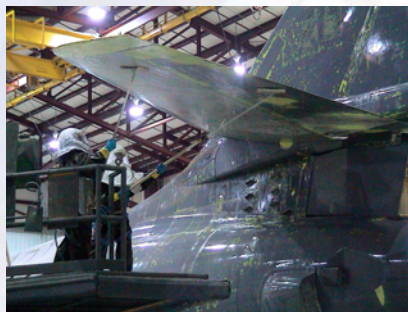
THE TAFB P2 TEAM SUCCESSFULLY IMPLEMENTED A NON-CHROMATED SURFACE TREATMENT (PREKOTE), WHICH ACHIEVES BETTER PAINT ADHESION AND SAVES $120,000 ANNUALLY.
