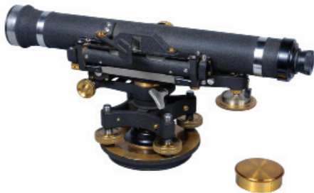
Tilting Level from Hoover Dam Collection (BOR)
