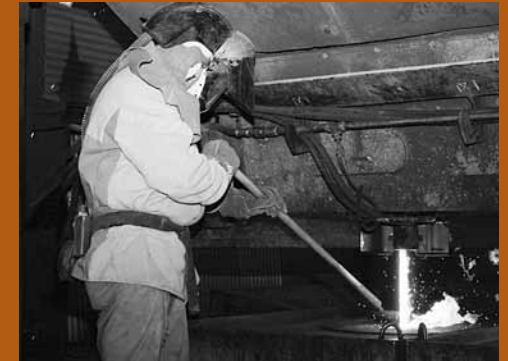
2011 Workplace Safety & Health Calendar: This worker at NuCor Steel in Seattle wears protective gear that includes flame-resistant clothing and a full-face respirator with a powered air filter.
