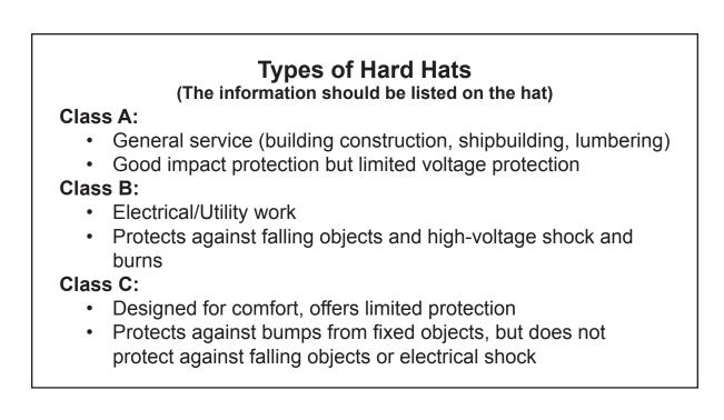
Hard hats must have a hard outer shell and a shock-absorbing lining that includes a headband and straps that suspend the shell from 1 to 1 1/4 inches away from the head. This provides shock absorption during an impact and ventilation during normal wear. Protective headgear must meet ANSI Standard Z89.1-1986 (Protective Headgear for Industrial Workers) or provide an equivalent level of protection (see Factsheet 5 for more information on ANSI Standards).
