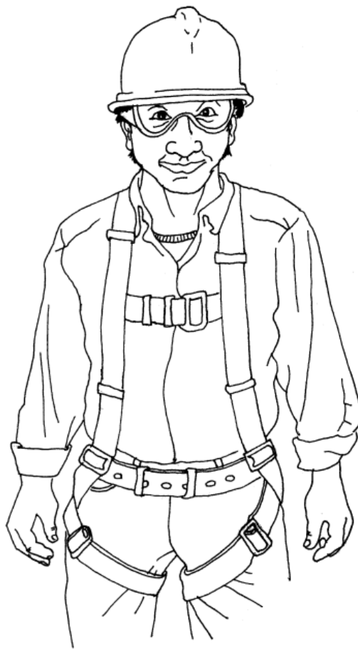
Safe Work: Worker is wearing a full body harness.
