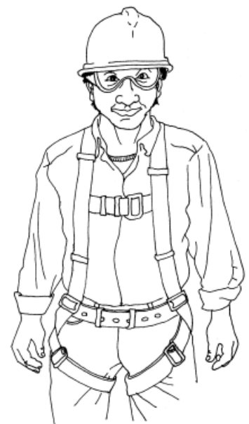
Safe Work: Worker is wearing a full body harness.
