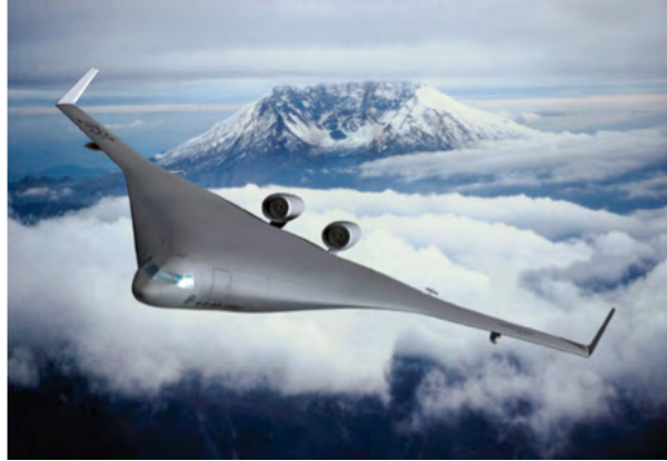
Figure 18. Hybrid wing-body aircraft have higher fuel-efficiency than traditional tube-and-wing designs for tankers and transports. Advances in integrated stitched-composite manufacturing technologies such as PRSEUS have enabled large, lightweight, high-stiffness panels at low cost.
