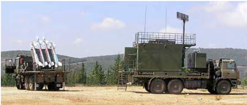
Advanced surface-to-air missile systems, such as the SPYDER that combines Python-5 EO/IR missiles with active radar-guided missiles, can provide highly capable area defense capabilities.
