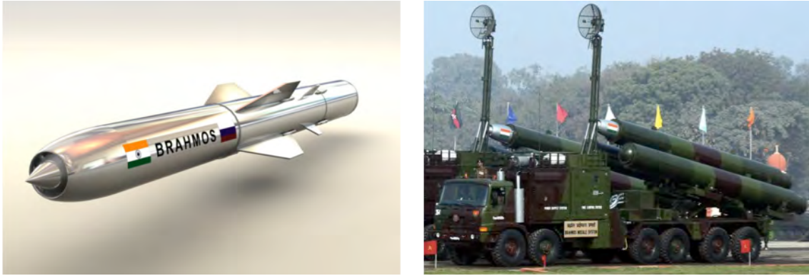
Figure 21. India and Russia have developed and fielded the Brahmos supersonic cruise missile reportedly capable of Mach 2.5 flight over ranges in excess of 250 km. Su-30 fighters are reportedly being modified to provide an air-launch capability, primarily for anti-ship and land attack roles.
