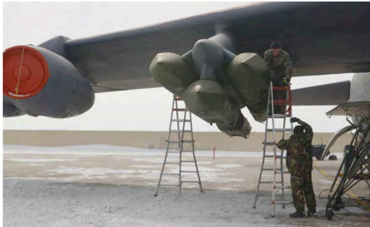
Continuing to strengthen the Air Force nuclear enterprise remains the top U.S. Air Force priority; here Airmen load AGM-129A advanced nuclear cruise missiles onto a B-52 at Minot AFB.
