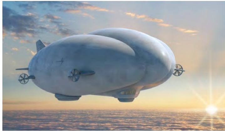
Figure 17. Hybrid airships that achieve part of their lift from buoyancy and part aerodynamically from forward flight can serve as highly efficient large-scale cargo airlifters for long-haul routes and in uncontested areas with unprepared landing sites.
