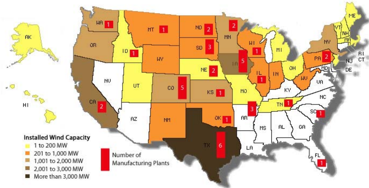
FIGURE 5 Installed wind capacity and location of blade, nacelle, and tower manufacturing plants, by state, March 2009
