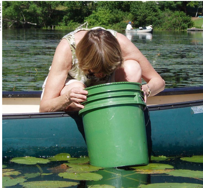
Homemade bucket scope gives Invasive Plant Patrollers a good view of underwater plants.
