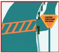
A Mobile Equipment Trainer and Safety Coordinator in Washington State sent in this idea; "Whenever Mobile Equipment and pedestrians are working in the same area, designated walkways for pedestrians should be established whenever possible. Equipment operators should use extreme caution when crossing walkways or working in areas where foot traffic is present. Best solution is to separate pedestrians from Mobile Equipment."
