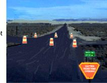
Where painting lines is either impractical or impossible, traffic cones or barrels are a good way to mark pedestrian crossings.
