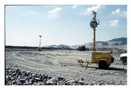
Provide adequate lighting for improved operator visibility during night time operations or when necessary. This allows drivers to better examine dump areas for cracks, inadequate berms, or other potentially hazardous conditions.
