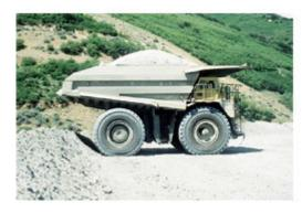
Grade dump-point areas so that trucks are backing up a slight grade to dump their loads. This helps drivers to control their trucks as they back up and keeps the dump area better drained, making it more stable. The dump berm should have a wide base to keep the truck back from the edge, which provides added stability. Drivers should avoid consistently relying on the berm to
