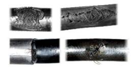
• Install abrasion protection such as spiral wrapping, sleeves, and guards.
