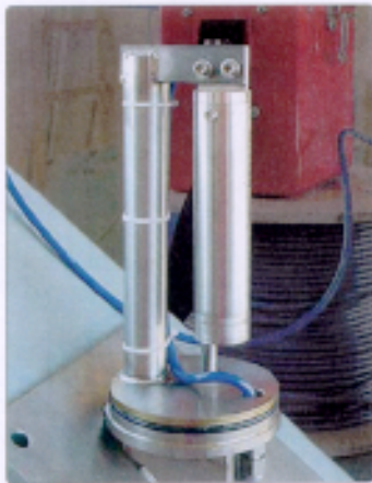
• Model 6350 installation using a custom mounting bracket designed for concrete face rock fill dam applications (shown with protective cover removed).
