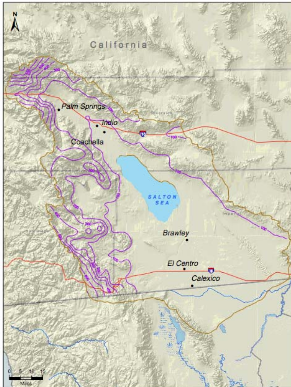
Figure 2.7: Contours of the mean annual precipitation \Delta W_p (in mm) over the Salton Sea Basin, as derived from accrued rainfall data between 1971 and 2000 provided by the PRISM Group, Oregon State University, http://www.prismclimate.org (Appendix A).
