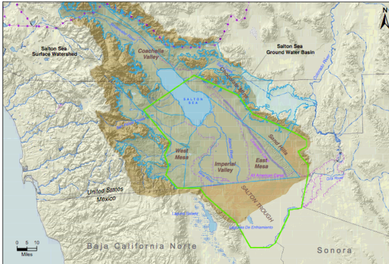
Figure 7.1: Map of the Salton Sea Basin showing the horizontal extent of the proposed 3D groundwater model domain (green), the overall Salton Sea watershed boundary (shaded), and the outlines of the recognized (US) groundwater basins (shaded with blue outlines).
