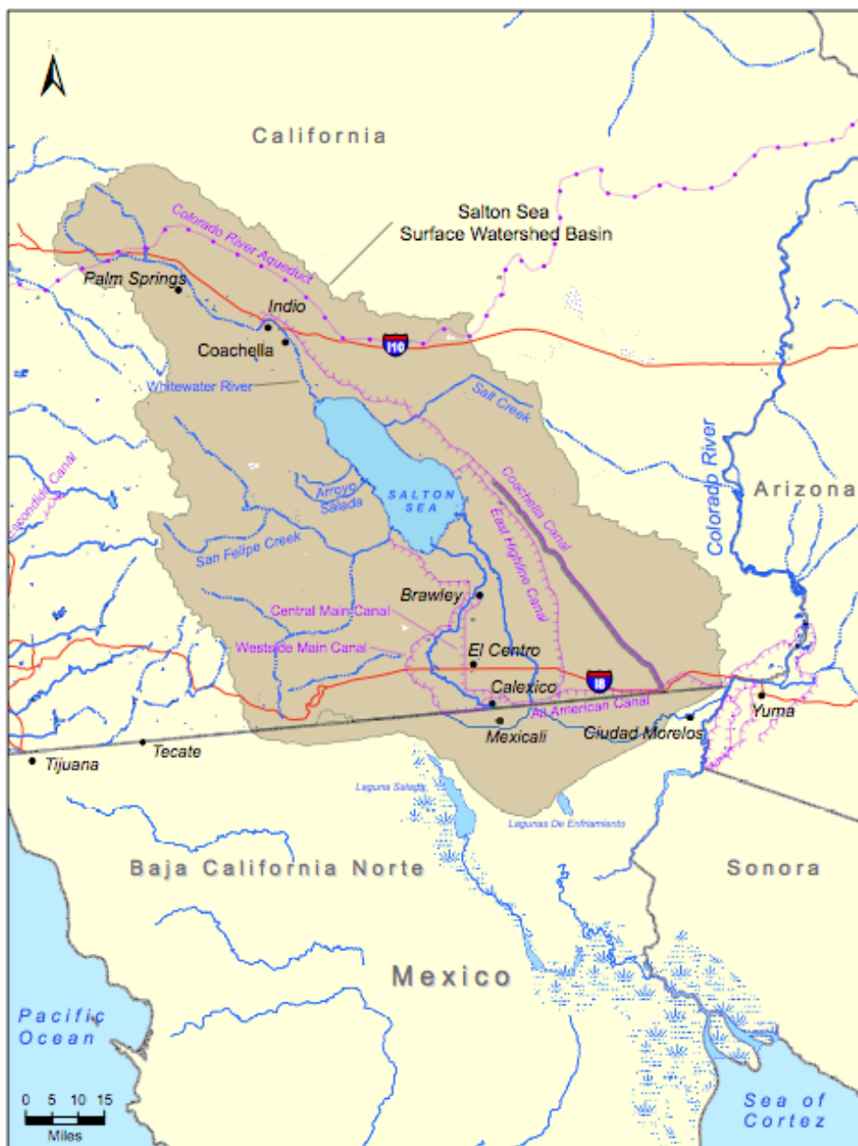
Figure 1.1: Map of the greater Salton Sea area in Southern California and Baja California Norte showing the Colorado River, imported water aqueducts (purple), and regional watershed basin (shaded, 8360 mi 2 , or 21,700 km 2 , in area). A thick gray line indicates the lined portion of the Coachella Canal.
