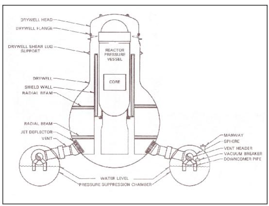
The above graphic shows a cross-section of a pressure suppression chamber, also known as a torus. The cross-section measures 29.6 feet wide. The chamber typically holds 790,000 gallons of water.
