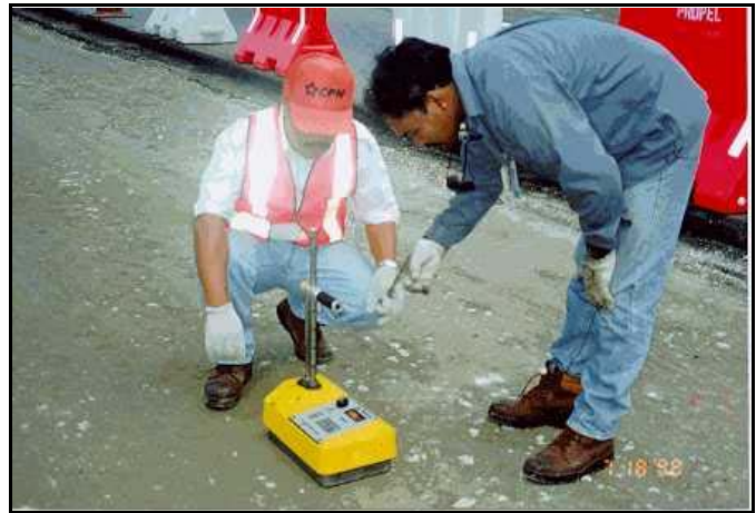
A typical moisture-density gauge in use.
