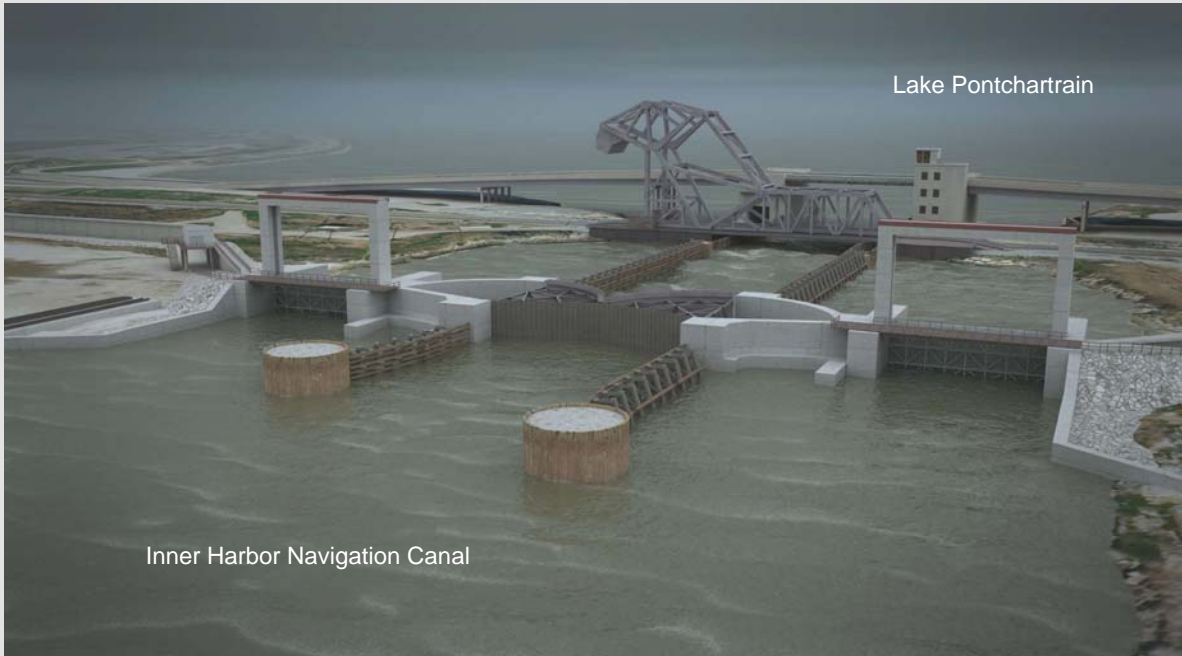
This conceptual illustration of the Seabrook Floodgate Structure shows the sector gate and the lift gates in the closed position, as it would look during a storm event. (USACE conceptual illustration)
