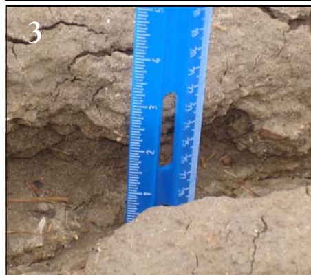
Photo 3 (above) shows the greatest erosion in the levee to be only three inches.
